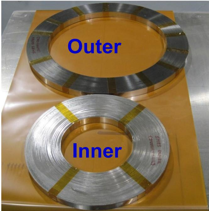
Made with ~210 meter of 12 mm ReBCO tape from SuperPower with SS tape between the turns (No. of turns = 258)
