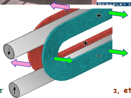
In cosine theta or conventional block coil designs, the coil module cannot move as a block. Therefore, Lorentz forces put strain on the conductor at the ends which may cause premature quench.
