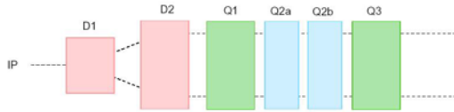
Figure 7: The dipole design concept developed here is suitable in the LHC IR Upgrade lattice proposed by CERN in the "Dipole First" option.
