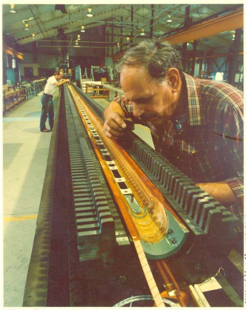
RHIC dipole coldmass during assembly
