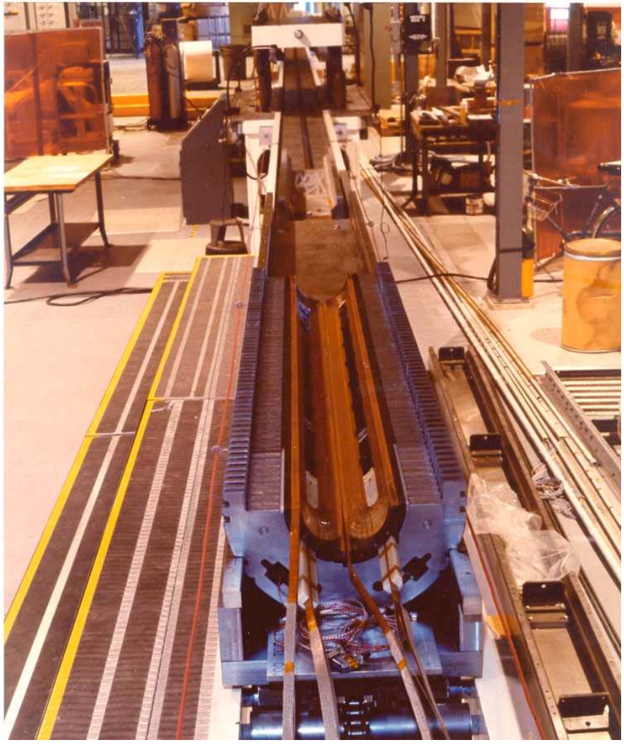
RHIC insertion quad coldmass during assembly
