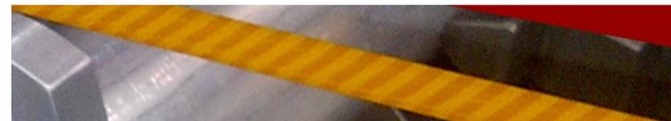
*Spirally wrapped with about 30% overlap between the adjacent Kapton layers*
