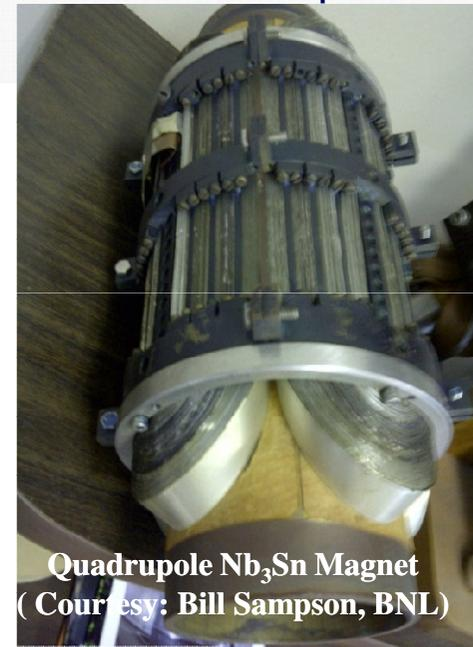
Quadrupole Nb<sub>3</sub>Sn Magnet
