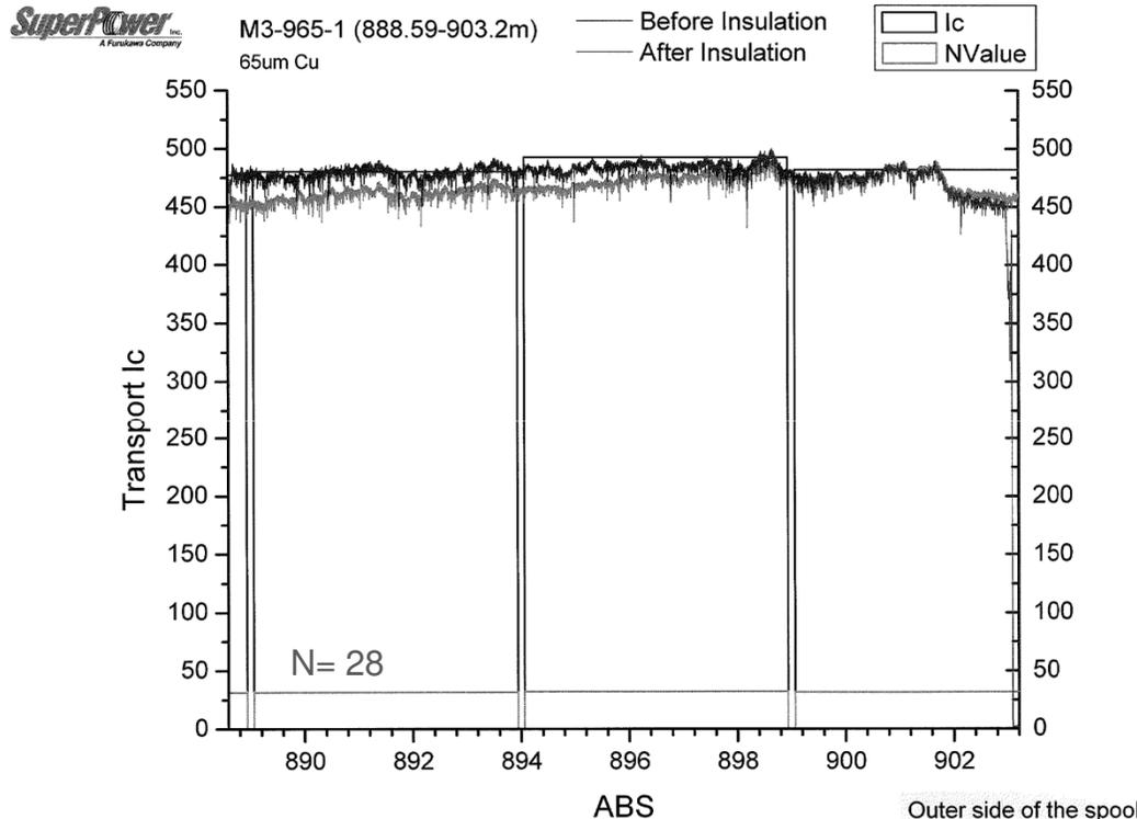
*Note : Transport current was tested at every 5 m at 77K; Ic is defined under the voltage criterion of 1μV/cm*
