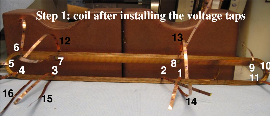
☞ voltage taps are installed in the smaller straight and critical bend sections of the innermost coil turn
