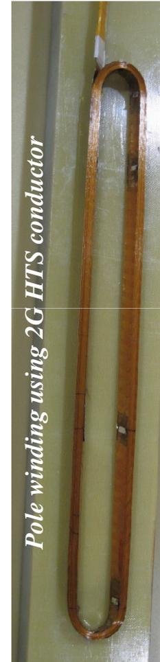
*This work is part of HTS Dipole STTR with Particle Beam Lasers Inc. (PI: Eric Willen)
