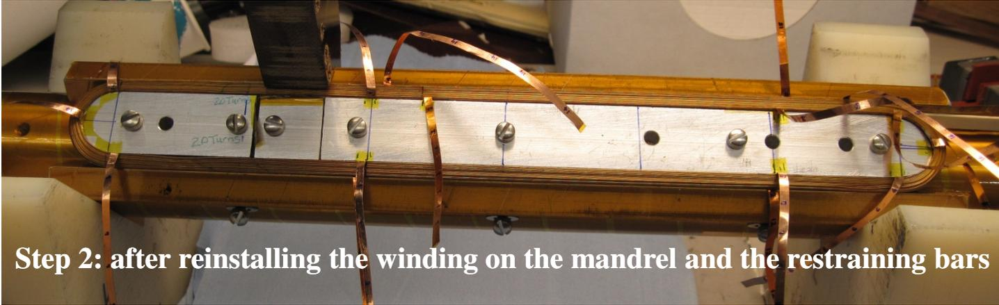
Step 2: after reinstalling the winding on the mandrel and the restraining bars
