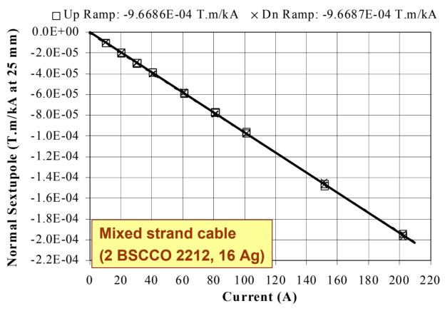
Difference between up and down ramp values is within measurement errors. Max field on conductor was only ~550 Gauss. Expect a relatively less measurement when the total current is high in an all HTS cable.
