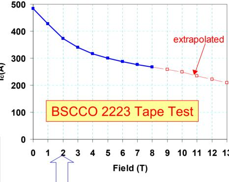
Measurements of "<u>BSCCO 2223</u> <u>tape"</u> wound at 57 mm diameter with applied field parallel ( $1\mu V/cm$  criterion)
