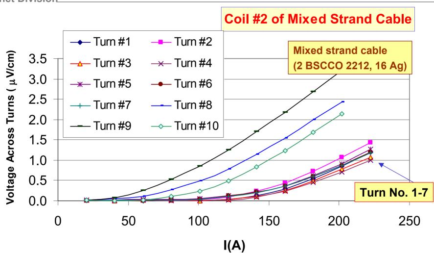
Turns No. 1-7 show an  $I_c$  close to the best measured in cable prior to winding.
