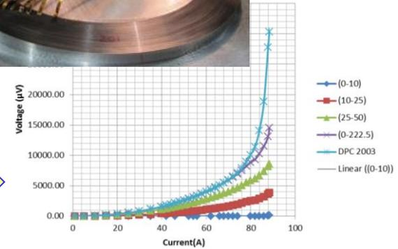
**Note: Thorough 77 K test of each pancake was an important part of a series for QA**
