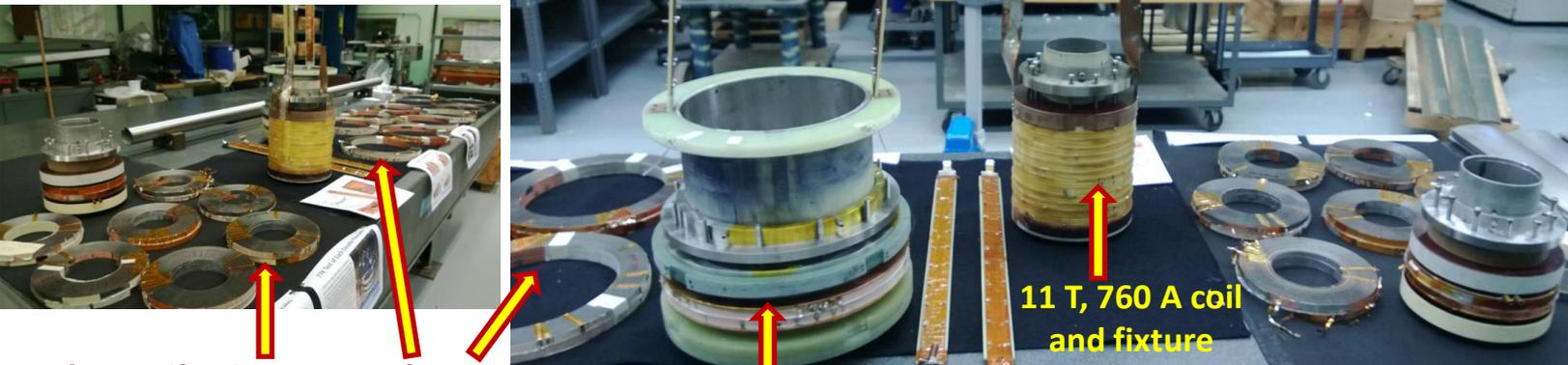
Pancake coils: inner and outer 77 K Test Fixture for outer 11 T, 760 A coil and fixture
