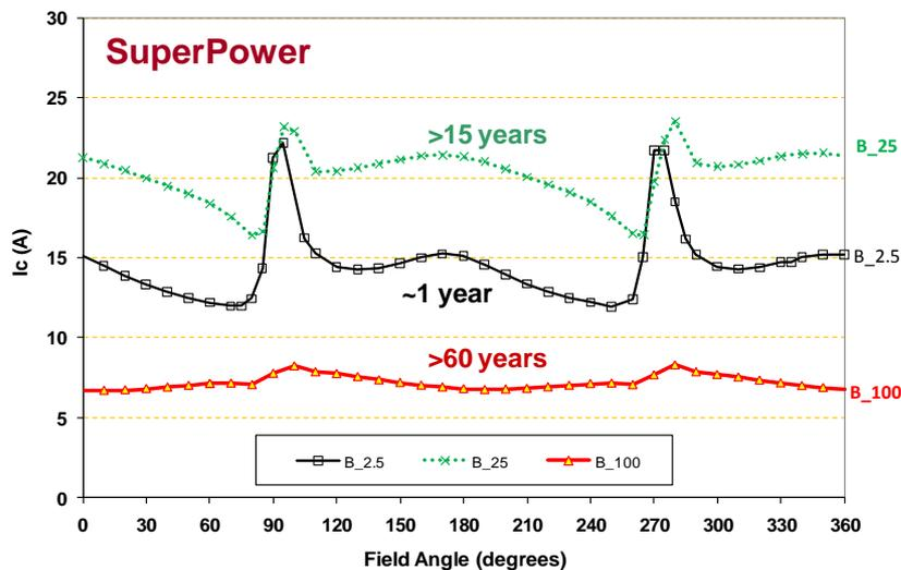
Ic Measurements of SuperPower and ASC at 77K in field of 1T
