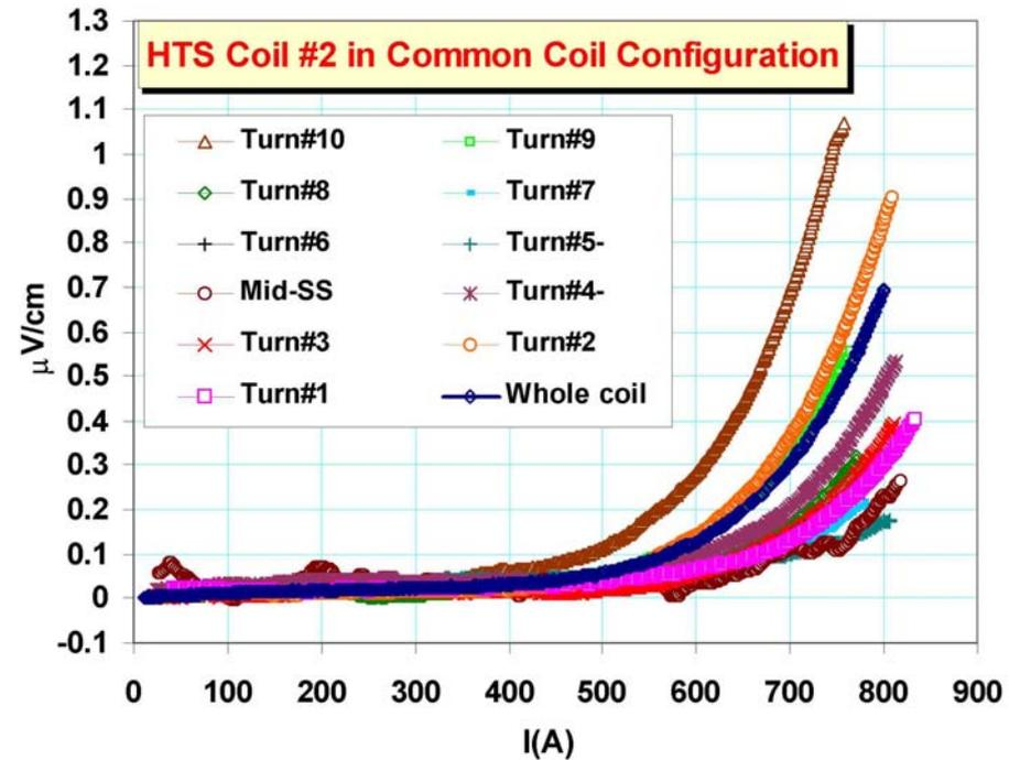
Measurements in HTS Magnet DCC002 at 4.2 K
