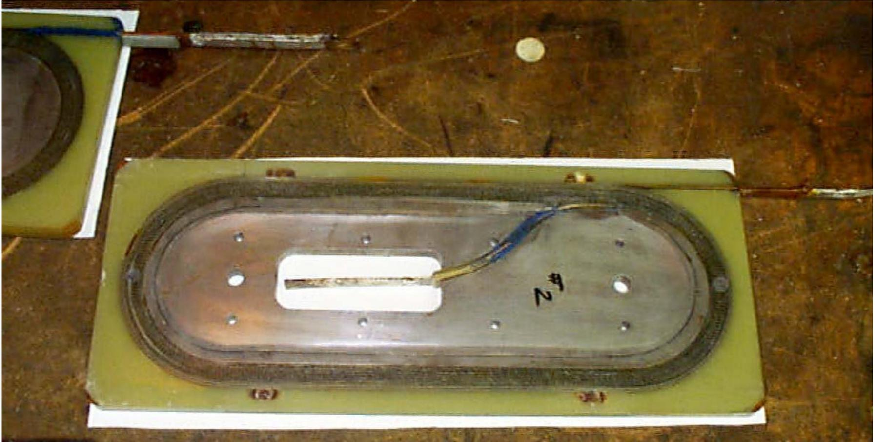
Vacuum impregnated coils made with the “react and wind” technique.
