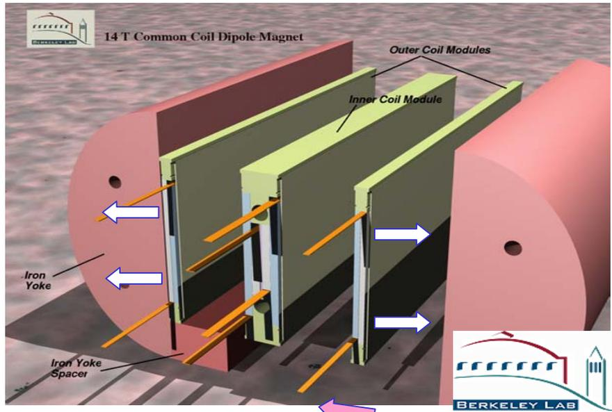
In cosine theta designs, the geometry is such that coil module cannot move as a block. These forces put strain on the conductor at the ends and may cause premature quench. The situation is somewhat better in single aperture block design, as the conductors don't go through complex bends.
