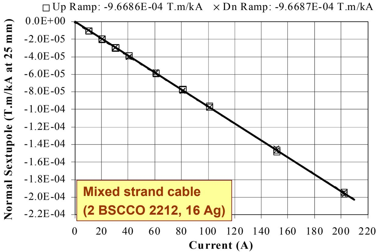
Difference between up and down ramp values is within measurement errors.
