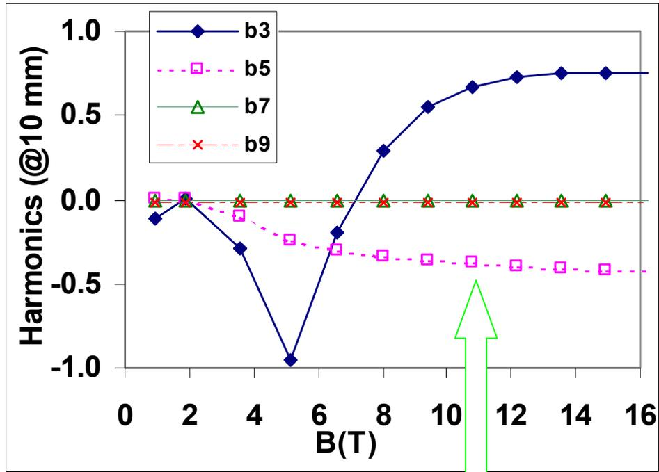
Low saturation induced harmonics up to 15 T with a single power supply
