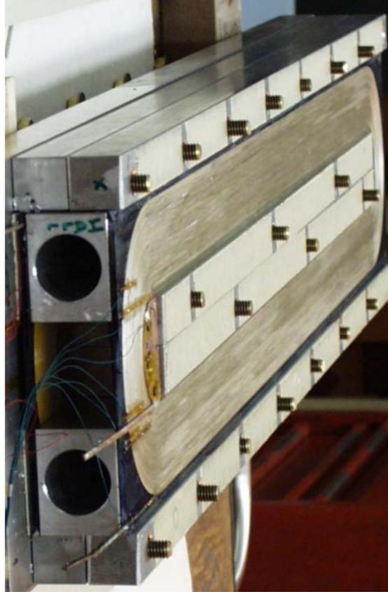
Two HTS tape coils in common coil configuration
