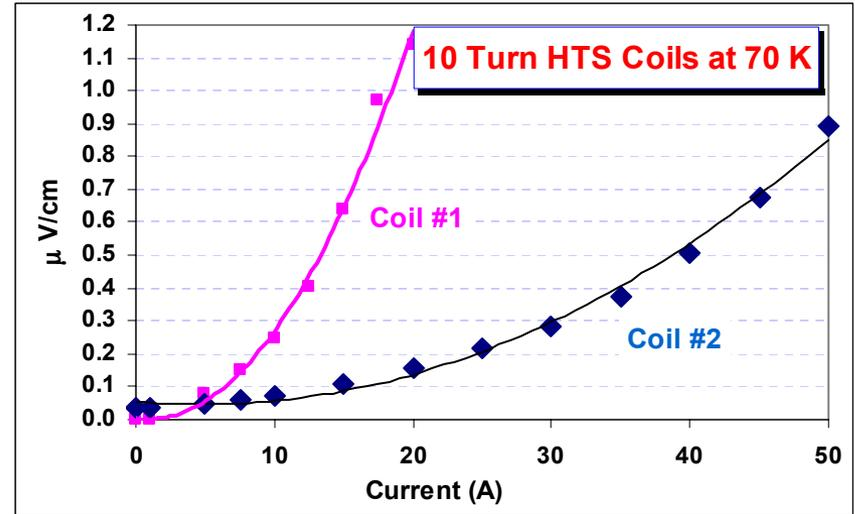
The HTS cables were from two different batches. They behaved differently:
