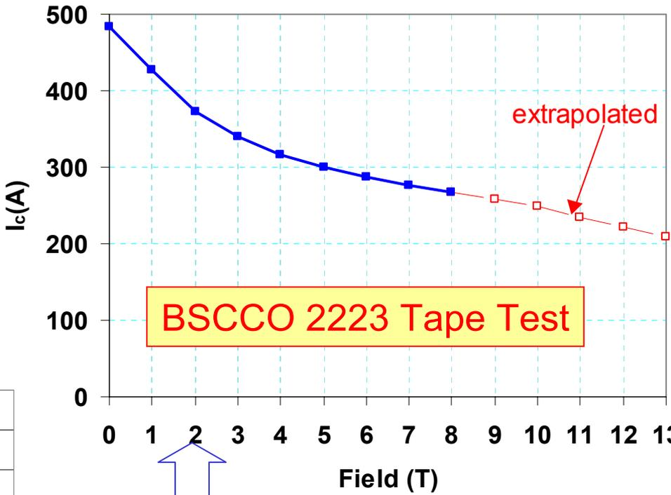
Measurements of "BSCCO 2223 tape" wound at 57 mm diameter with applied field parallel ( $1\mu V/cm$  criterion)
