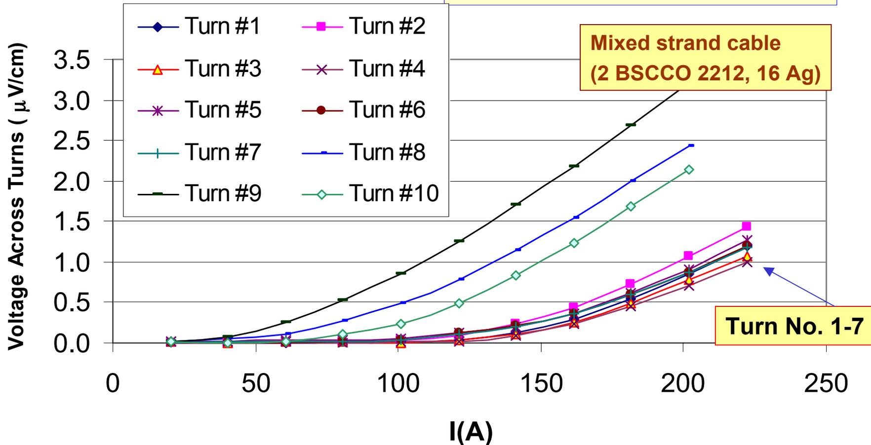
Turns No. 1-7 show an  $I_c$  close to the best measured in cable prior to winding.
