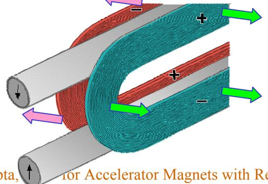
We must check how far we can go in allowing such motions in the body and ends of the magnet. This may significantly reduce the cost of expensive support structure. Field quality optimization should include it (as was done in SSC and RHIC magnet designs).
