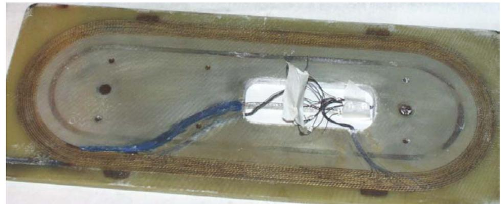
Conductor friendly racetrack coil with large bend radius
