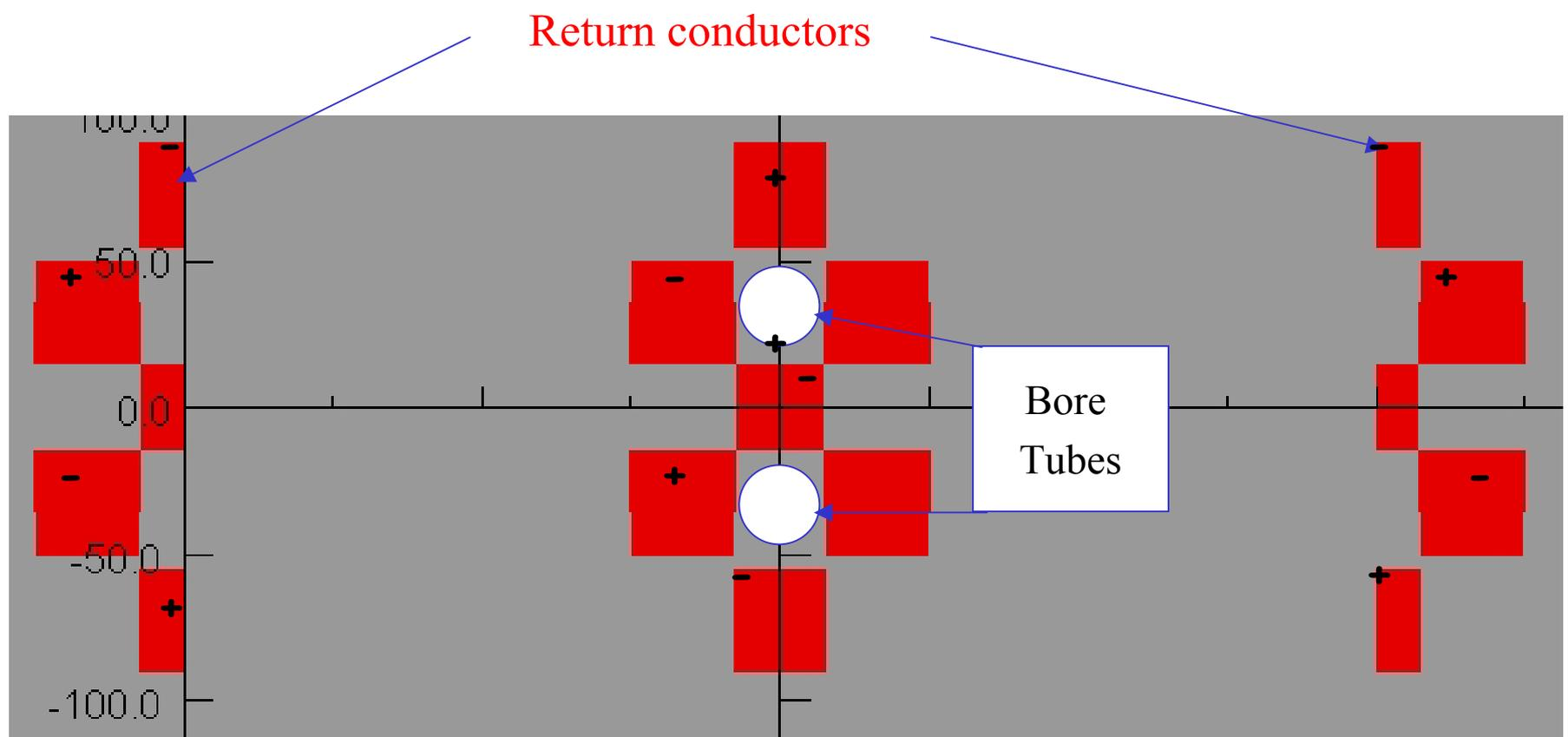
(simple racetrack coils with large bend radii allow the use of HTS)
