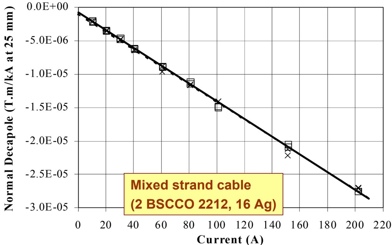
Difference between up and down ramp values is within measurement errors.
