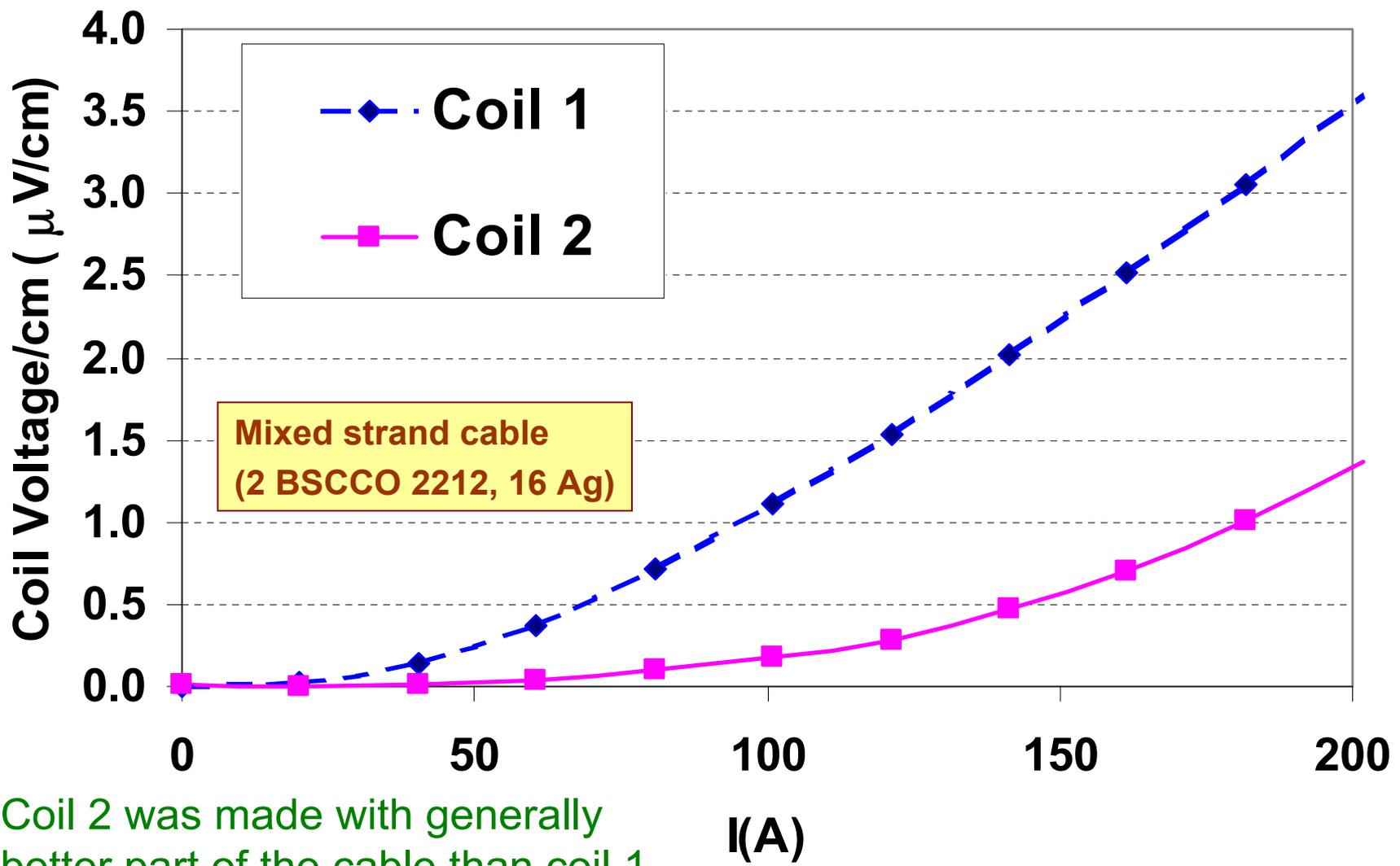
Coil 2 was made with generally better part of the cable than coil 1
