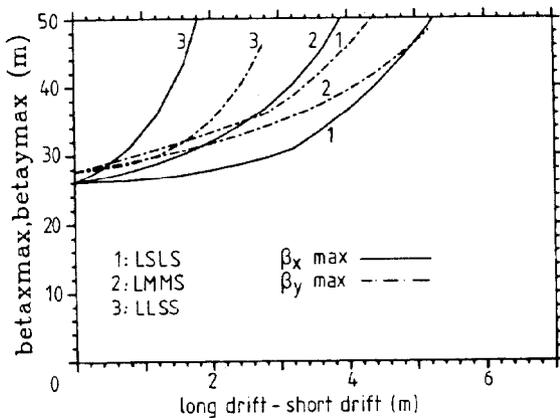
Fig. 4. Betafunction peak values versus long-short drift difference.
