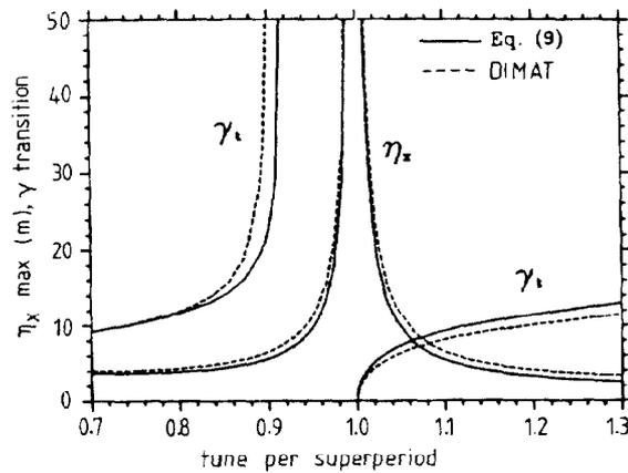
Fig. 1. Peak dispersion and  $\gamma_t$  as a function of tune in a missing magnet lattice.
