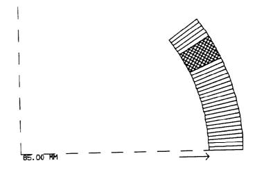
Figure 1: Cross section of the coil for RHIC insertion quadrupoles.
