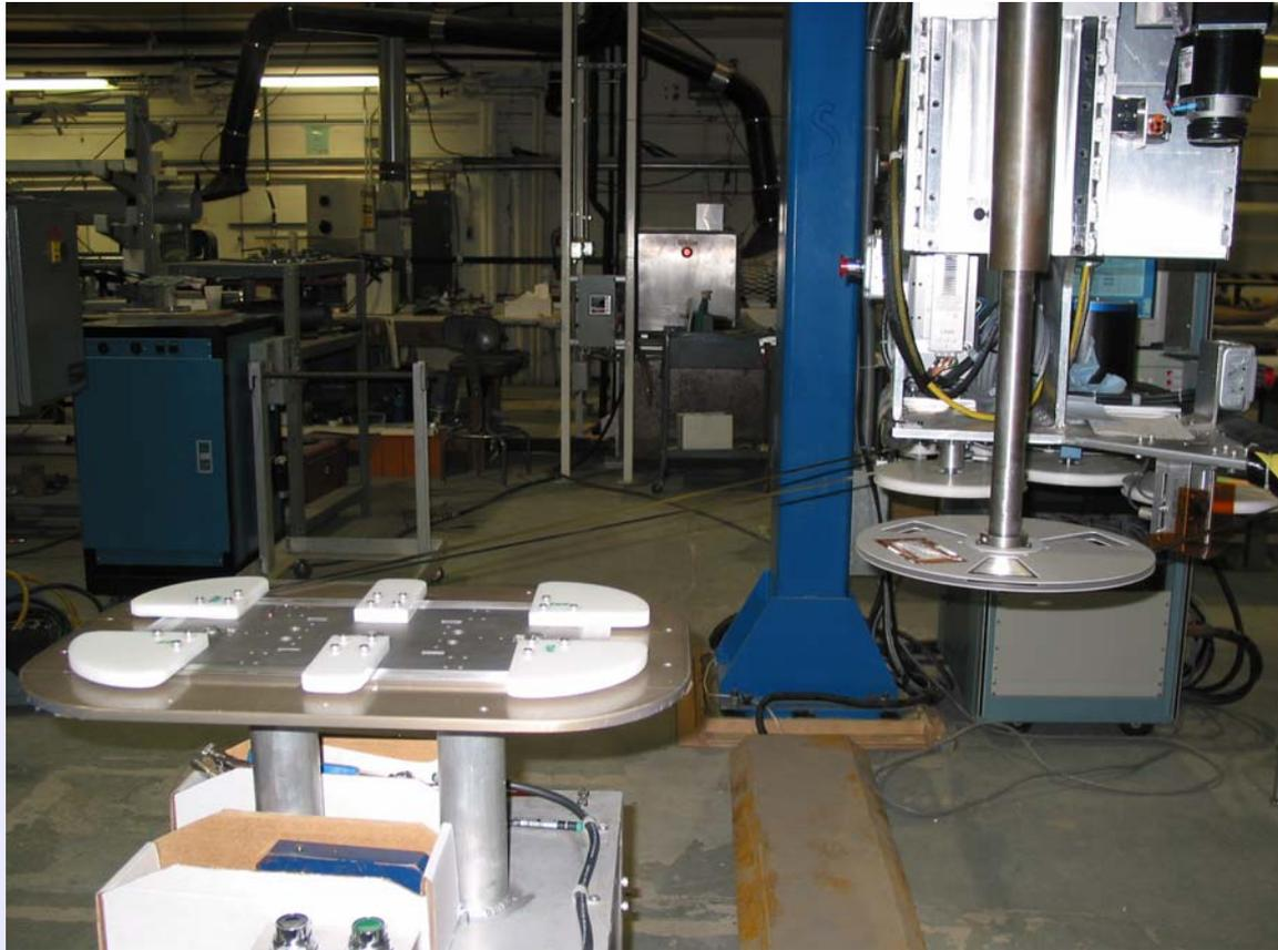
FRIB/RIA Coils being wound with S.S. tape over HTS
