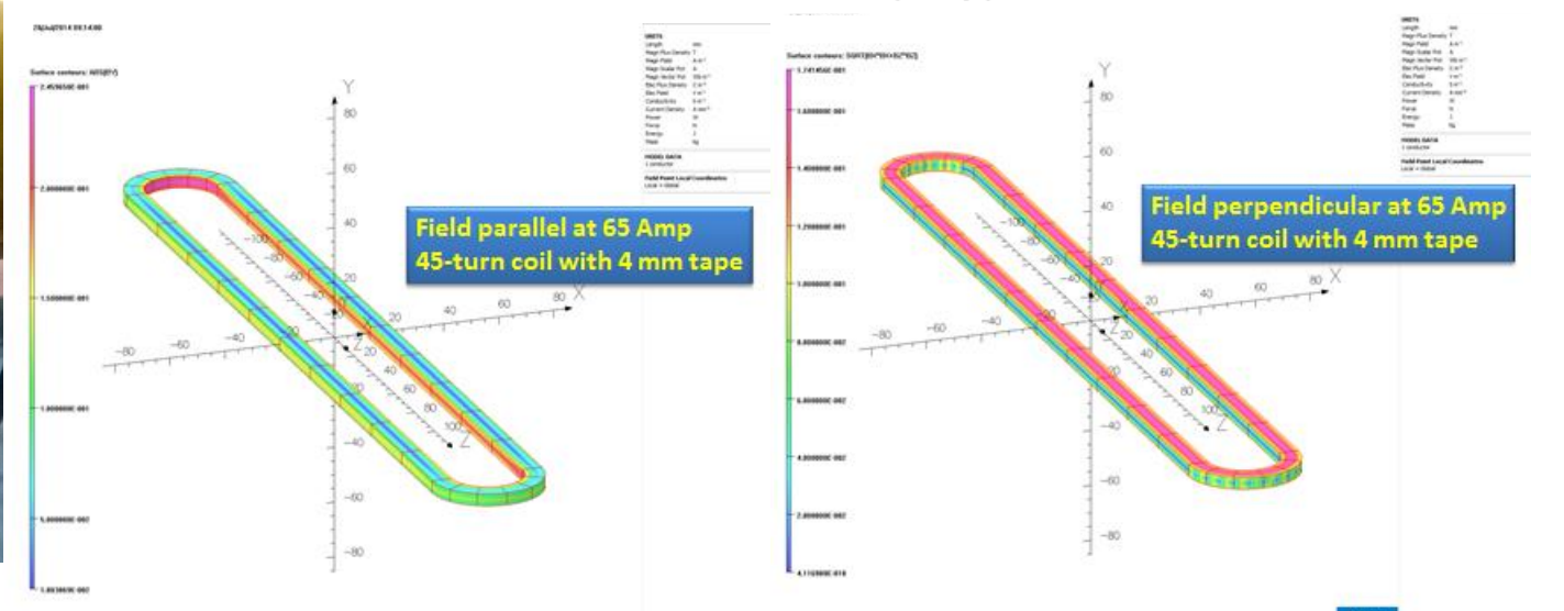
Computed magnitude and field perpendicular component at 65 A, superimposed on the 4 mm wide 20-turn coil
