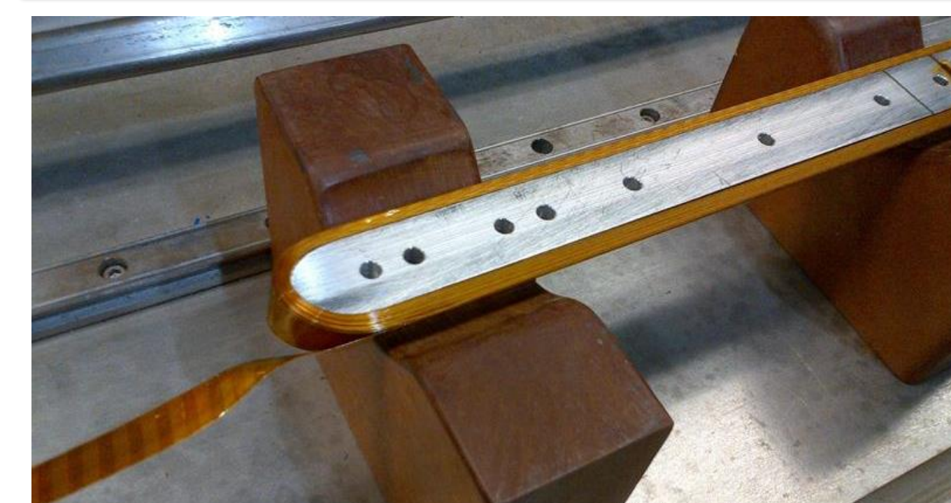
The 20-turn pole winding after fabrication. The 12 mm wide HTS tape conductor with its Kapton CI wrap is visible on the left.
