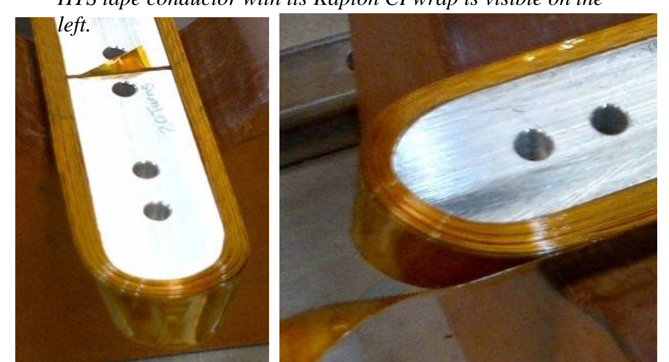
The 20-turn pole winding after fabrication. The 12 mm wide HTS tape conductor with its Kapton CI wrap is visible on the left.
