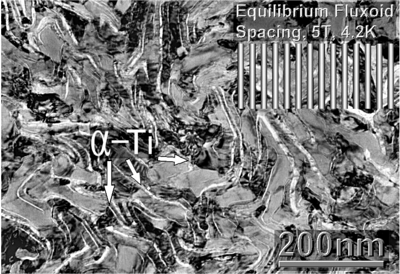
High critical current density microstructure in a conventionally processed Nb-Ti microstructure. Courtesy: P.J. Lee (University of Wisconsin-Madison)
