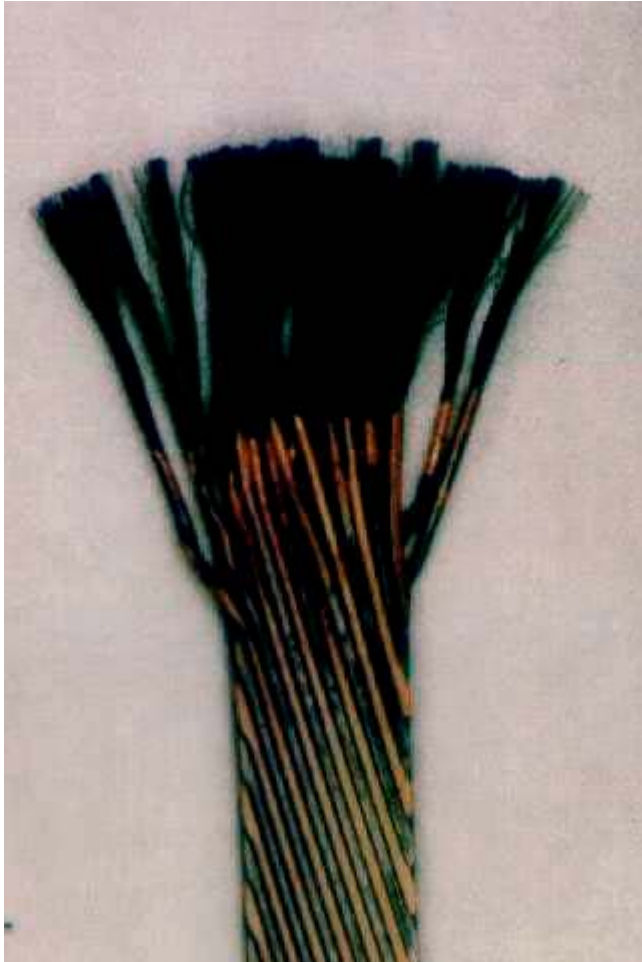
Filaments in an actual cable (Filament size in SSC/RHIC magnets: 6 micron)
