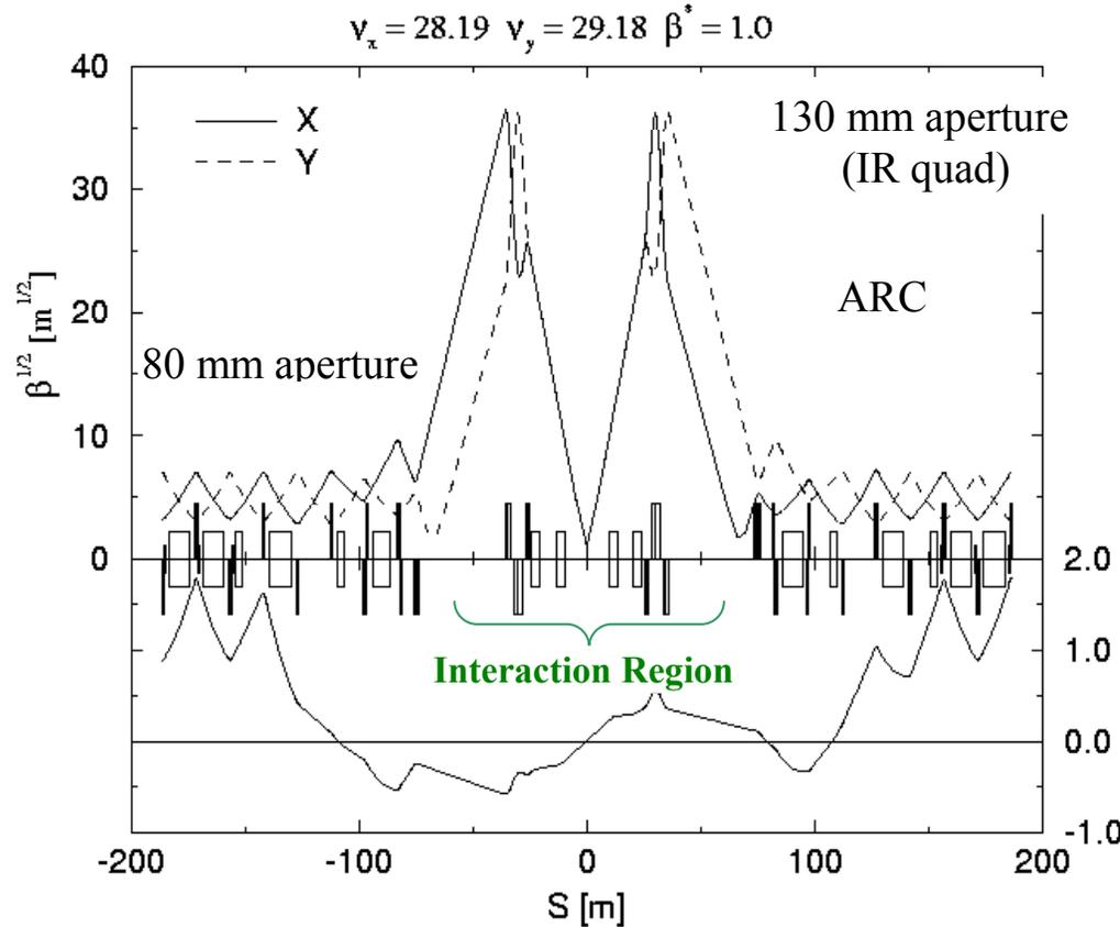
Compare the beam size versus magnet aperture in RHIC :
