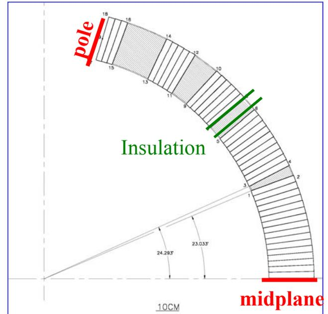
Geometric: Start with a larger than required shim and midplane cap. Then adjust it, as required without changing the cross-section of the cured coil. One can also adjust the layers of wedge/cable insulation, if needed. These three parameters can adjust the first two allowed harmonics and pre-stress or cable insulation. This approach was used extensively in various RHIC magnets.
