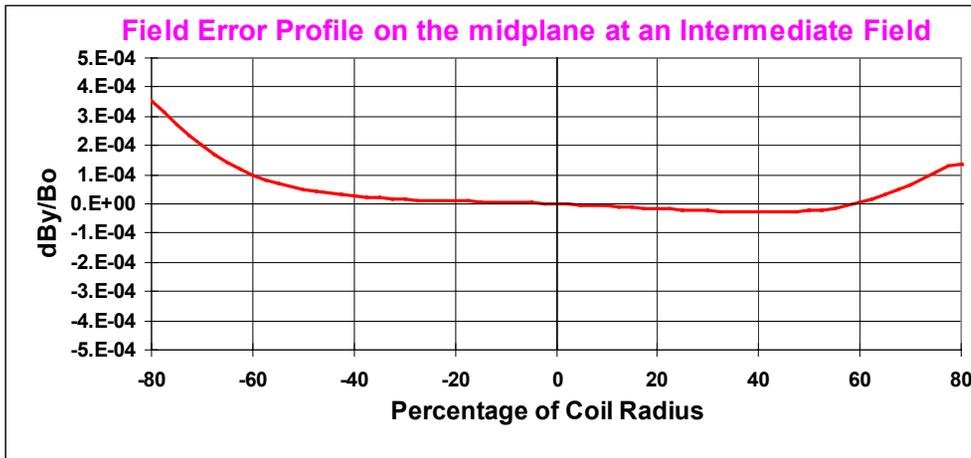
Note: Field errors are within  $10^{-4}$  at 60% of coil radius and  $\sim 4 \cdot 10^{-4}$  at 80% radius.
