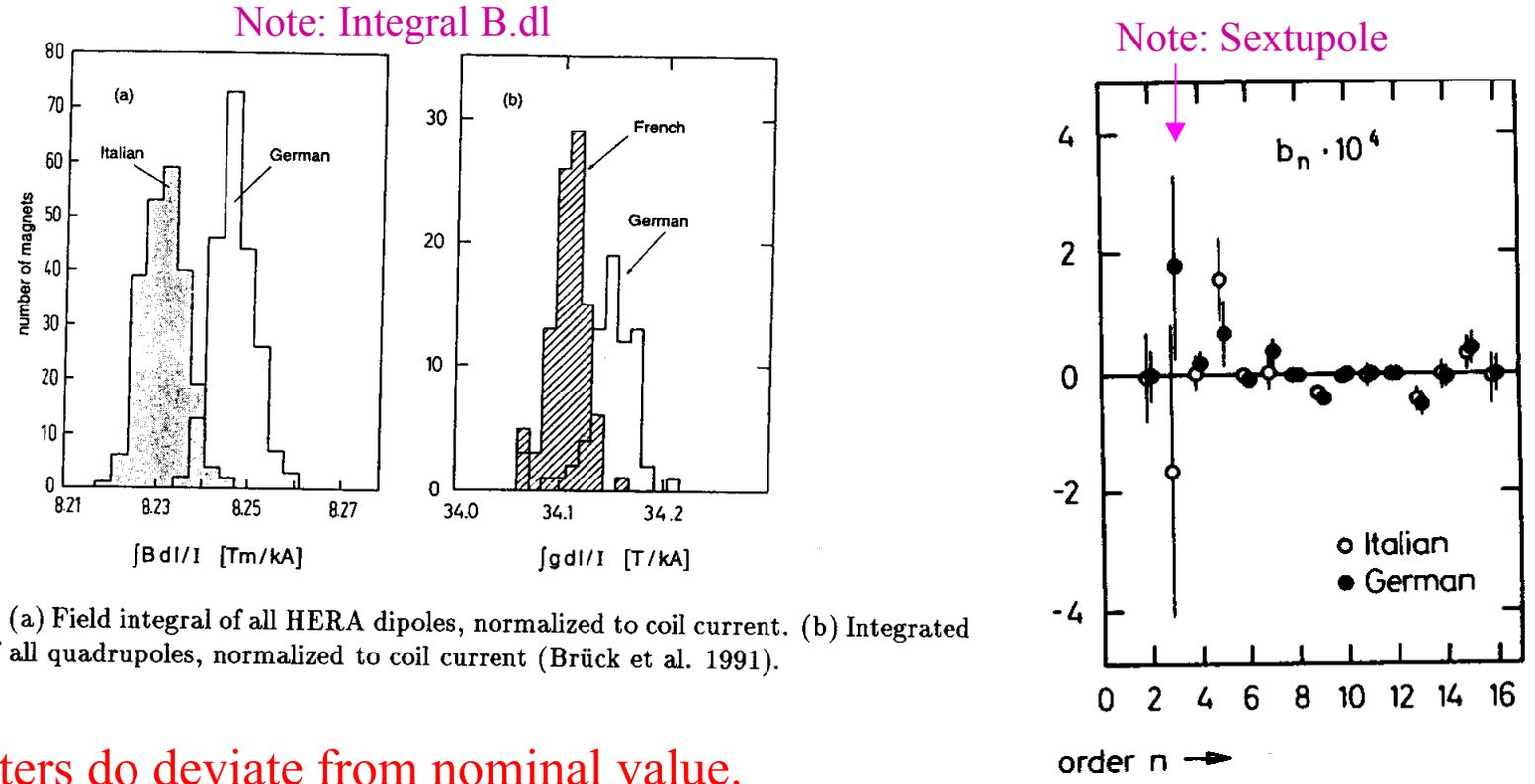
Figure 5.5: (a) Field integral of all HERA dipoles, normalized to coil current. (b) Integrated gradient of all quadrupoles, normalized to coil current (Brück et al. 1991).
