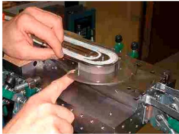
Figure 3. Applying laminar springs, ribs and plates to inner winding of Nb 3 Sn.
