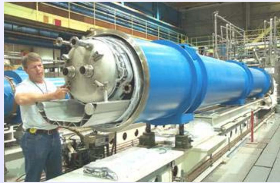
RHIC dipole coldmass during assembly
