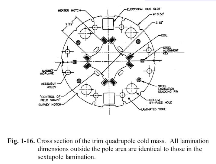
**Fig. 1-16.** Cross section of the trim quadrupole cold mass. All lamination dimensions outside the pole area are identical to those in the sextupole lamination.
