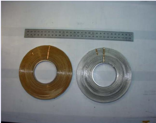
Two double pancake NMR coils, one with kapton insulation and the other with stainless steel.
