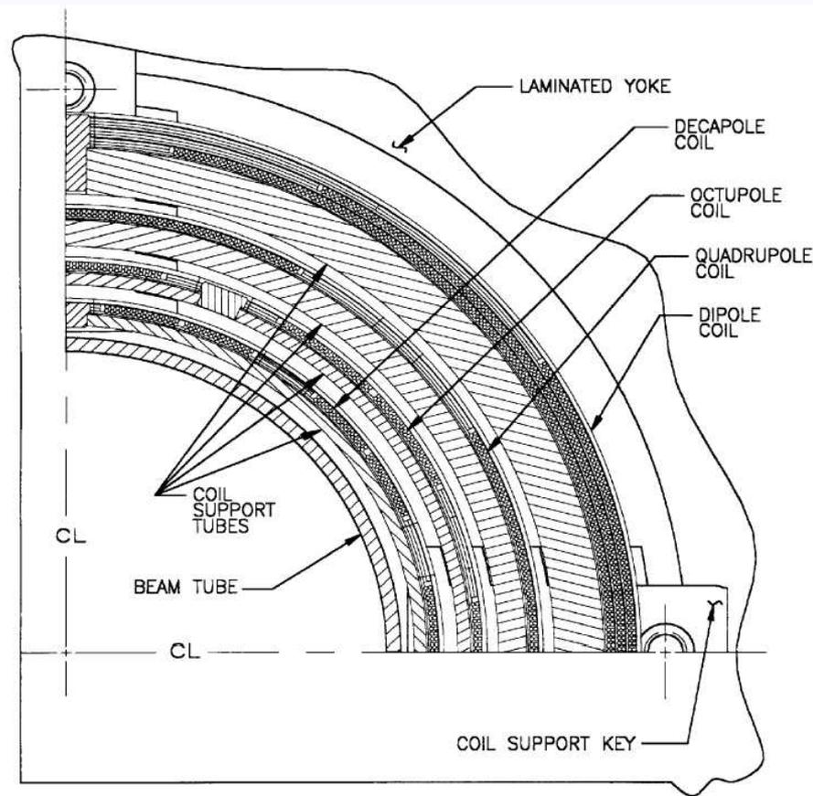
Fig. 1-11. Arc corrector coil cross-section (beam tube i.d. = 69 mm).
