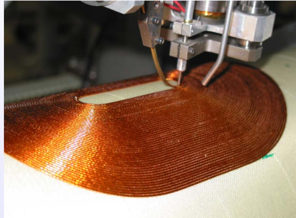
Superconducting wires are directly wound on the tube
