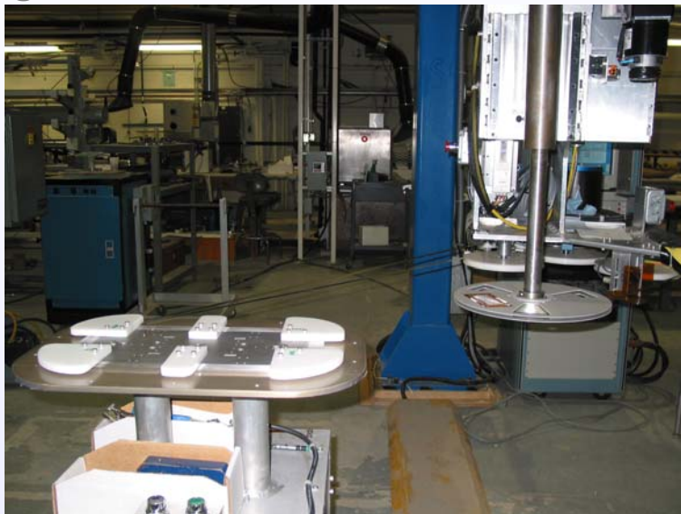
HTS coil winding with SS tape insulator
