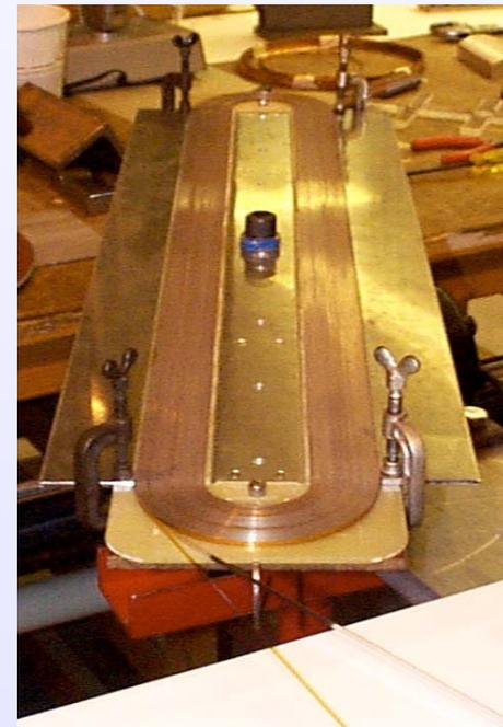
**HTS Test Coil for an Accelerator Magnet**
