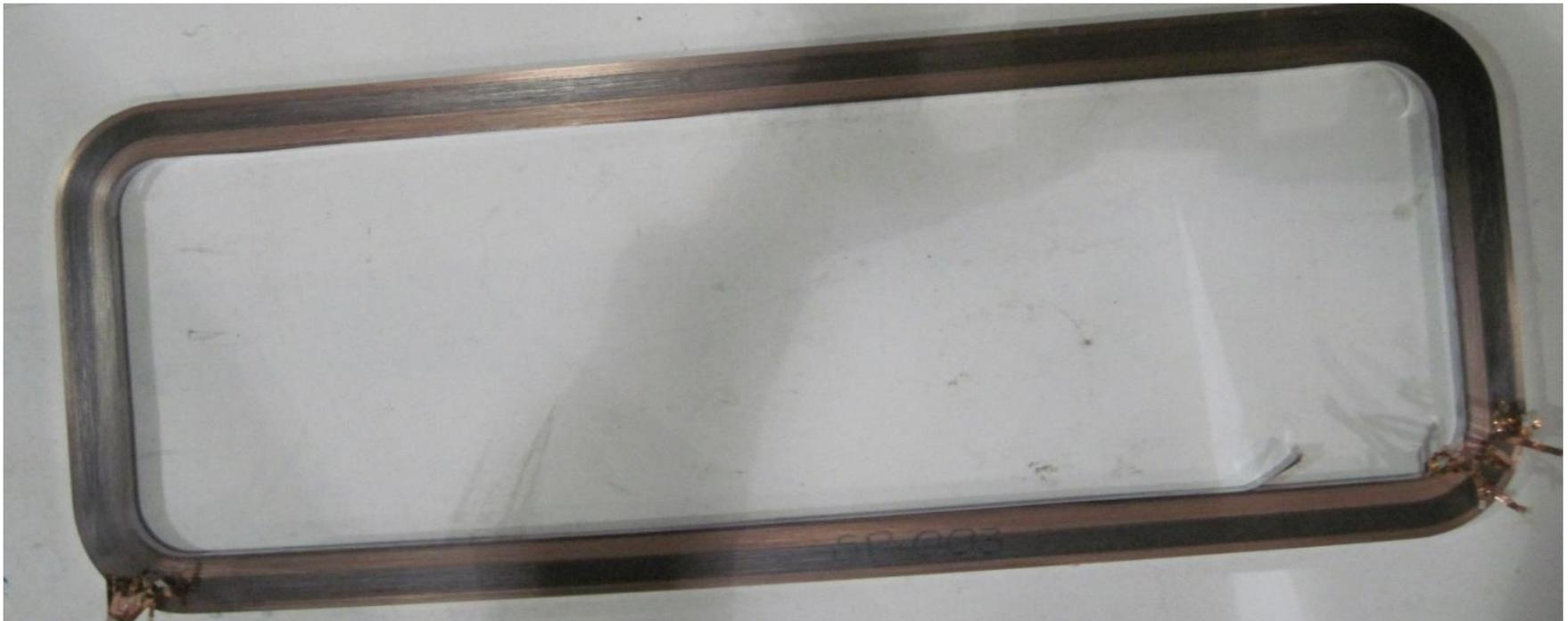
Fully wound coil with SuperPower tape with one splice
