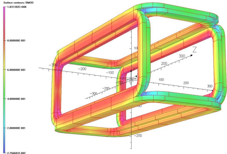
**Design (38 K): SP coils ~210 A & ASC coils ~310 A (equal Amp-turns).**
