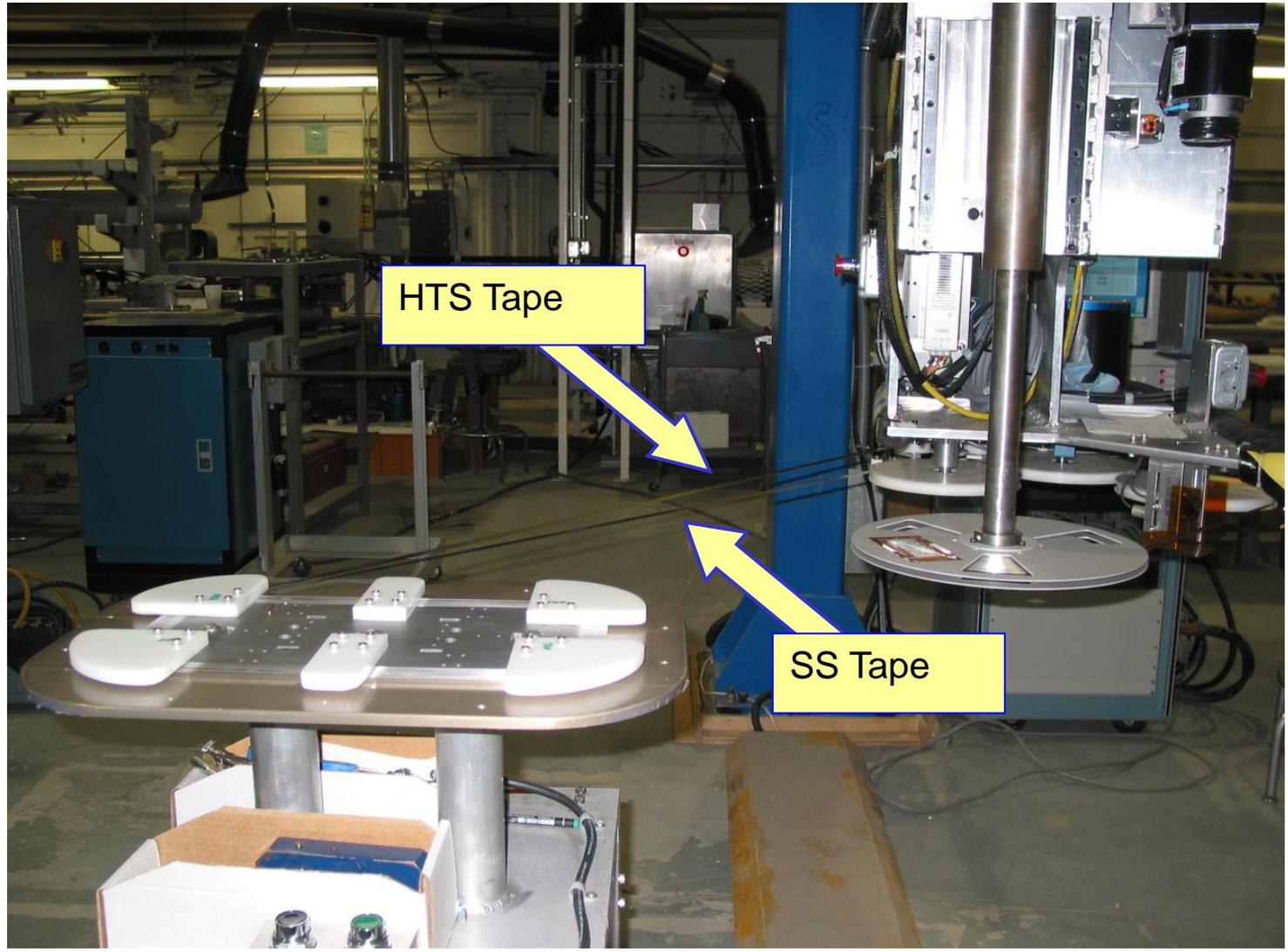
*A coil being wound in a computer controlled winding machine*
