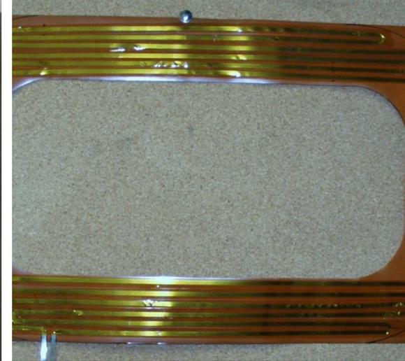
**Stainless steel tape heaters for energy deposition experiments**
