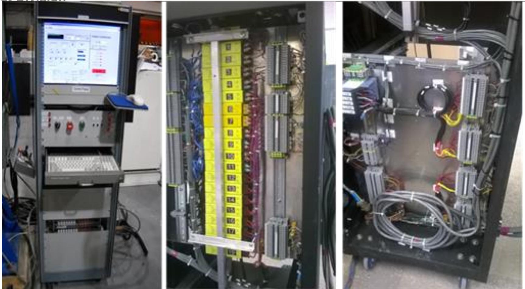
**Detects onset of pre-quench voltage at  $< 1\text{mV}$  and with isolation voltage  $> 1\text{kV}$  allows fast energy extraction**
