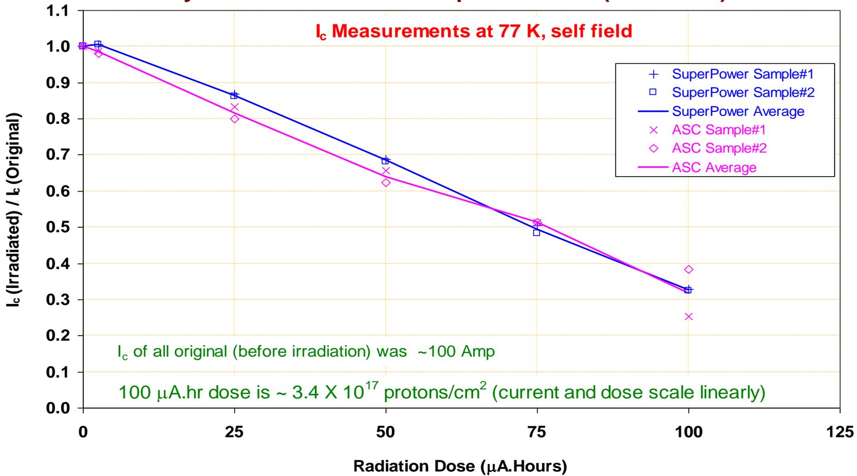
**SuperPower and ASC samples show very similar radiation damage at 77 K, self field**
