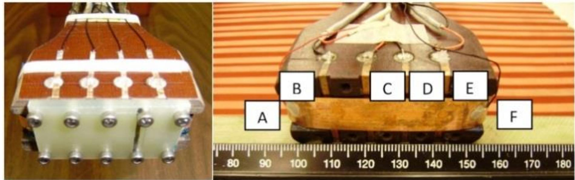
**B** Sample Holder for in-field  $I_c$  Measurements at BNL
