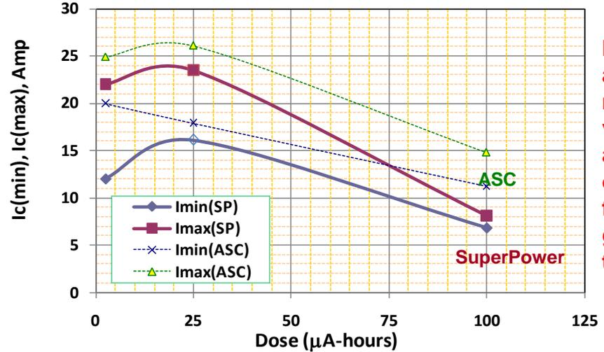
Ic Measurements of ASC at 77K in background field of 1T
