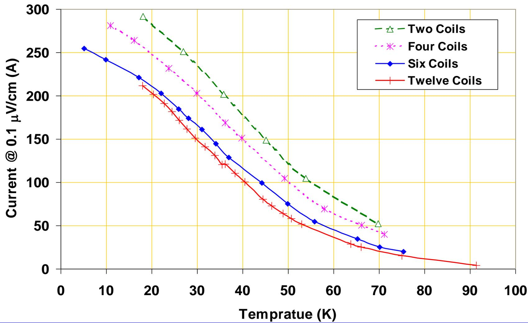
**Operation over a large temperature range- only possible with HTS**
