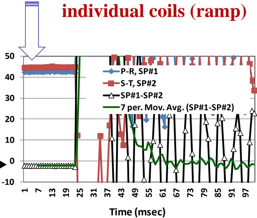
**Small quench detection threshold (2 mV) kept during the ramp by monitoring difference voltage**
