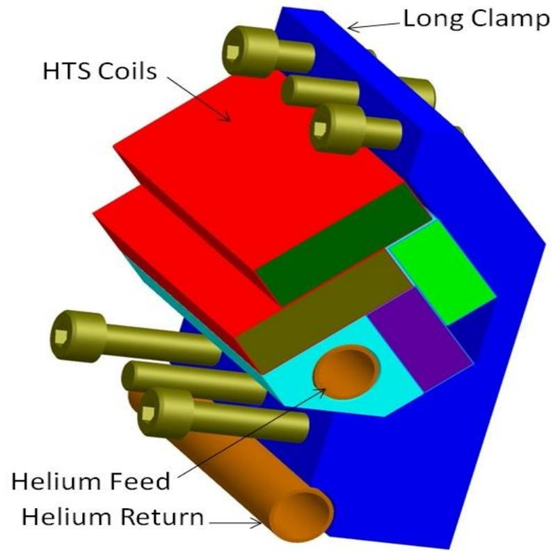
**Partial View of Clamped Coil**
