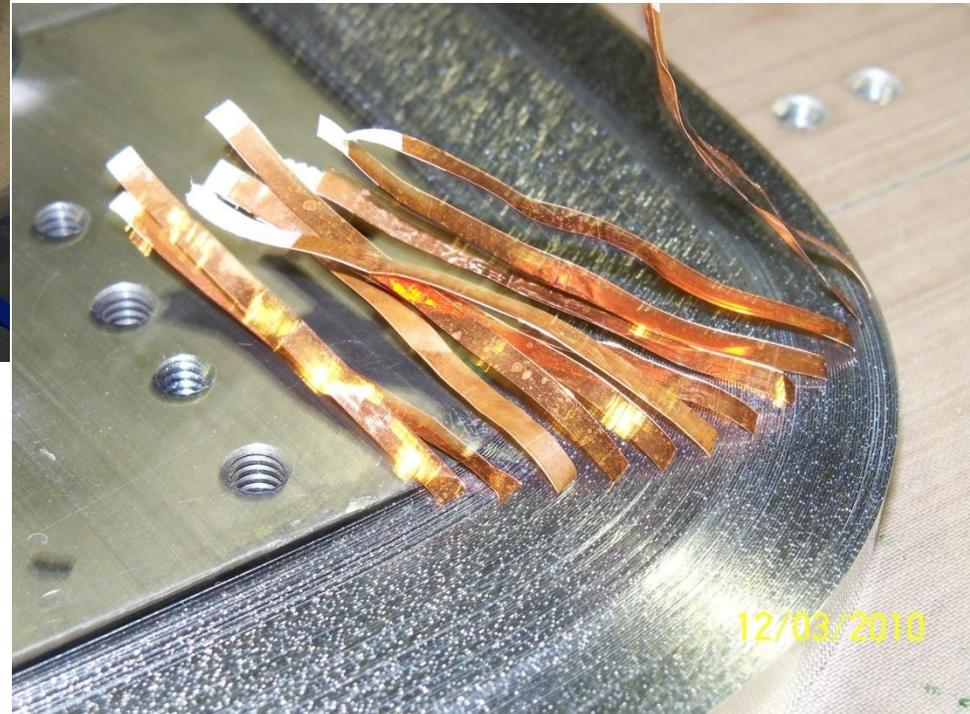
Voltage taps are placed generally after every 25 turns and also on either side of an internal splice
