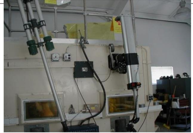
**$I_c$  Measurements of SuperPower and ASC at 77K in field of 1T**
