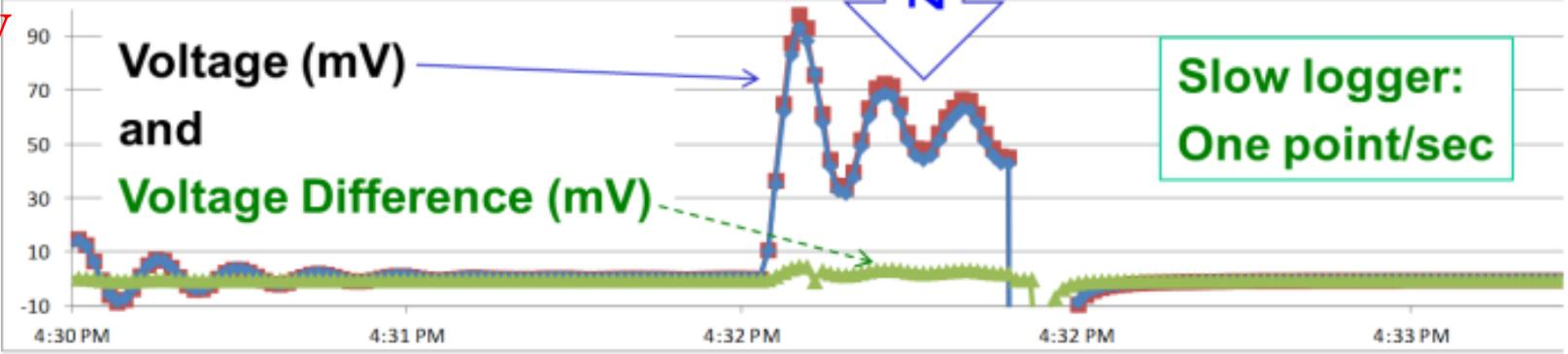
Event (Quench?) while ASC Coils were held at 382 A (design: 310 A) at ~50 K (design: 38 K)
