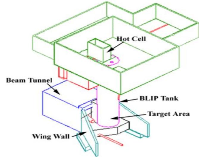
Figure 3. BLIP Beam Tunnel and Target Schematic
