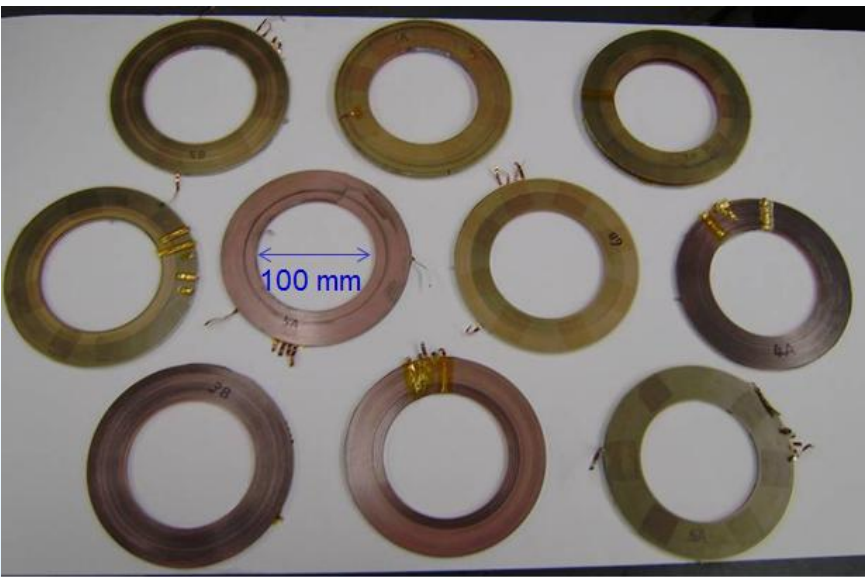
Proof That A Large Number of 2G HTS Coils Can be Built and Tested without Degradation
