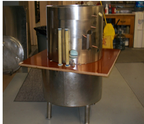
Figure 9: Solenoid in test cryostat with shield in place for magnetic measurements at design field at 77 K.
