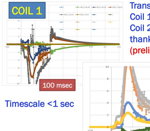
Transport current zero after 4 msec. Coil 1 voltage may be inductive but Coil 2 voltage may be real resistive, thanks to screening currents... (preliminary but very interesting)
