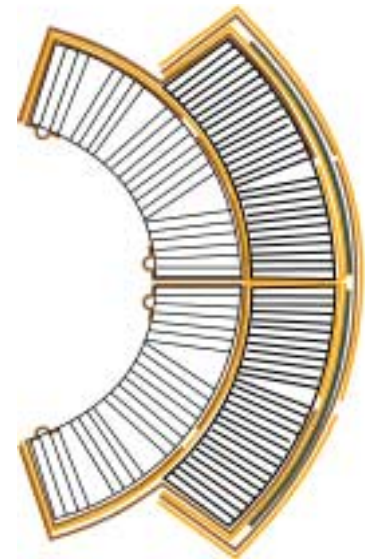
Kapton Insulation on SSC Coil
