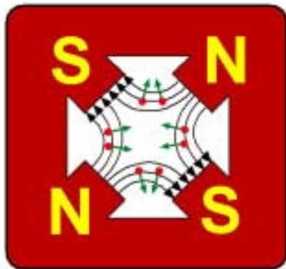
Rotated Normal Quad Horizontal focusing- "Focusing"
