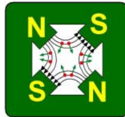
Normal Quad Vertical focusing - "Defocusing"
