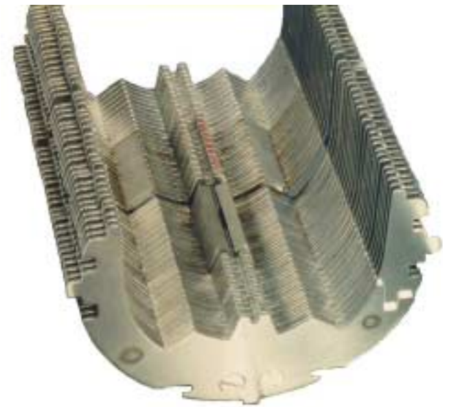
Collar pack (Nitronic 40 stainless steel) from an SSC prototype dipole
