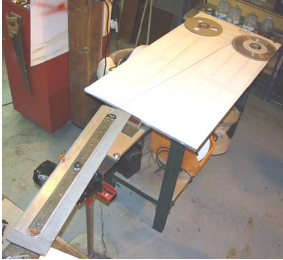
A coil being wound with HTS tape and insulation.
