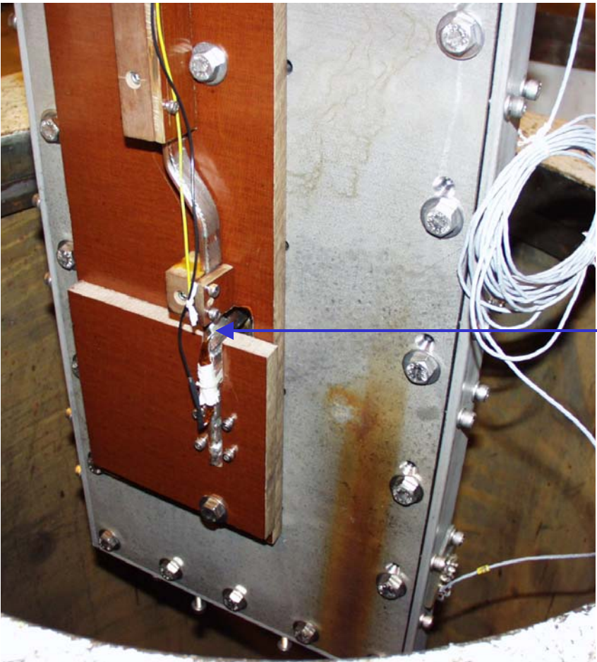
Splice for a single coil test (perpendicular splice take out the current to outside lead)
