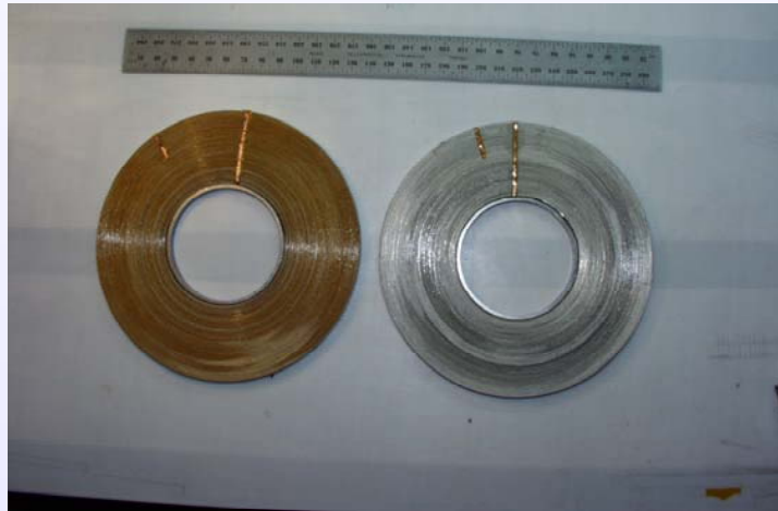
Two coils, one with kapton insulation and the other with stainless steel.
