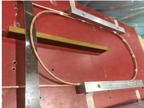
Cable bent and lifted (as per the design of DCC017)
