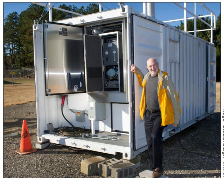
Above: BNL scientist Ernie Lewis and one of the mobile SeaTainer units now installed aboard the *Horizon Spirit*, a 272-meter cargo ship that will take atmospheric measurements during a yearlong cloud/climate study.
