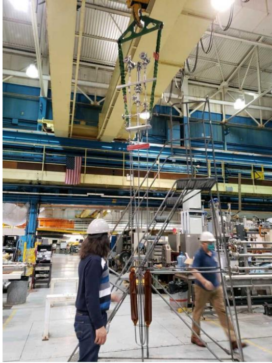
Figure 13 – Sample ready for installation into magnet bore.
