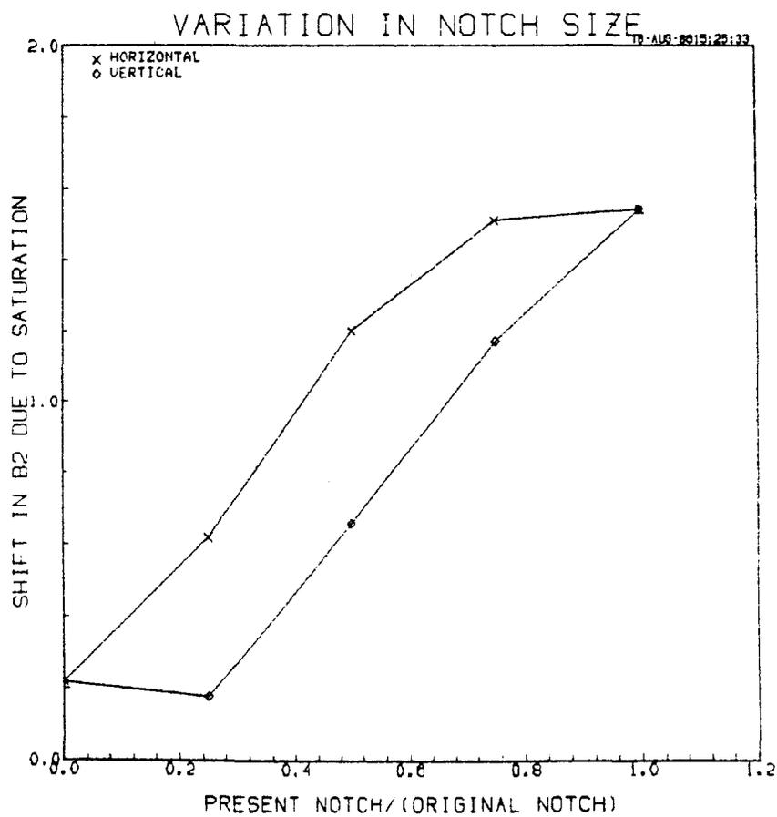
Fig 4. The effect of varying the size of the pole notch on the shift of sextupole harmonics due to iron saturation. The vertical size is held constant when the horizontal size is varied and vice-versa.
