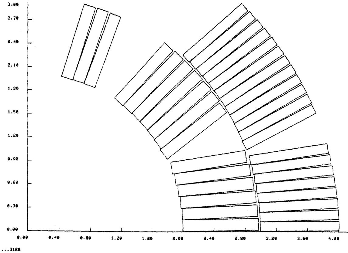
Fig 2(a). The details of coil structure on MDP for 1/r type current density distribution. The inner and outer layers of the coils are separated.
