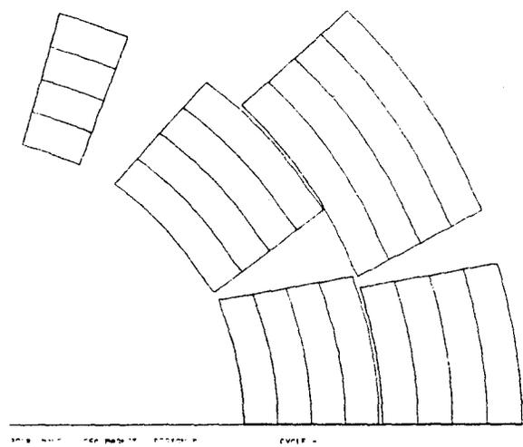
Fig 2(b). The details of coil structure on POISSON for 1/r type current density distribution. The inner and outer layers of the coils are separated.
