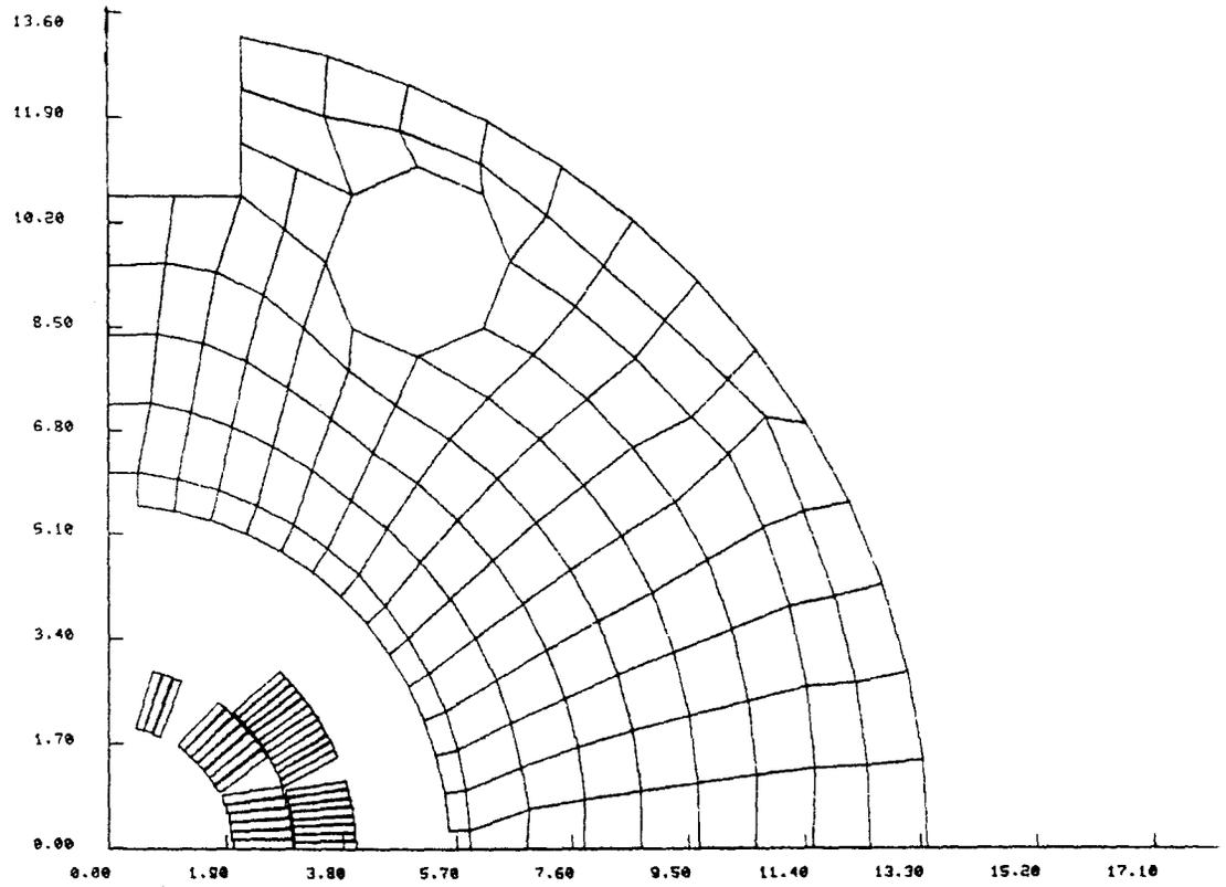
Fig 1(a). The Model of the SSC Design D Magnet on MDP.
