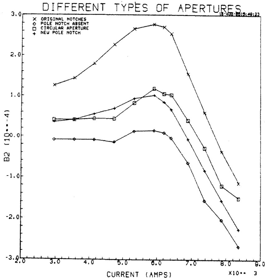
Fig 5(b). The sextupole harmonic for different types of aperture as computed by the code POISSON.
