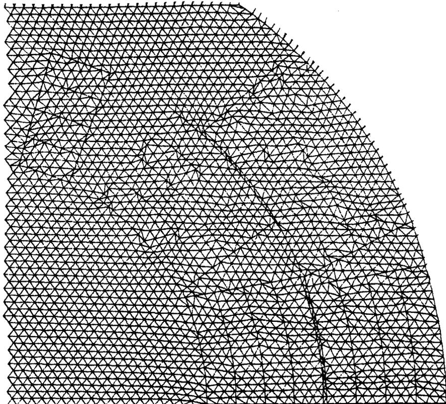
Fig 3(b). The mesh in the coil region. As appears in Fig 3(a) it is much denser than at any other place in our model.
