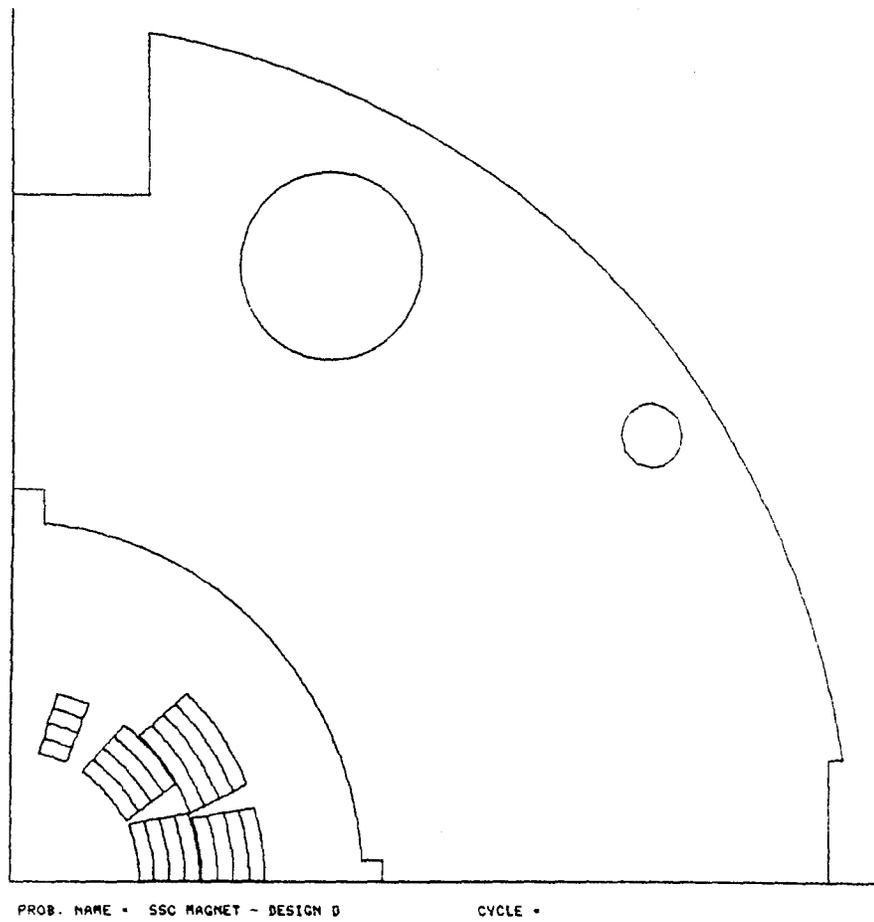
Fig 1(b). The Model of the SSC Design D Magnet on POISSON.
