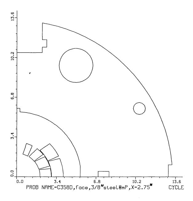
Fig 1. POISSON model for the proposed lamination
