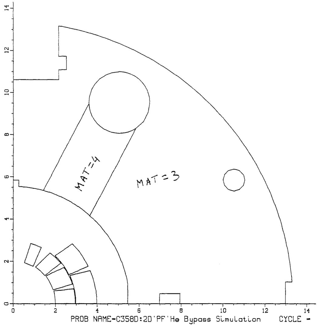
Fig 3. The use of MAT=4 at the cutout to describe the iron of different packing factor than the one (MAT=3) used in the rest of the iron.
