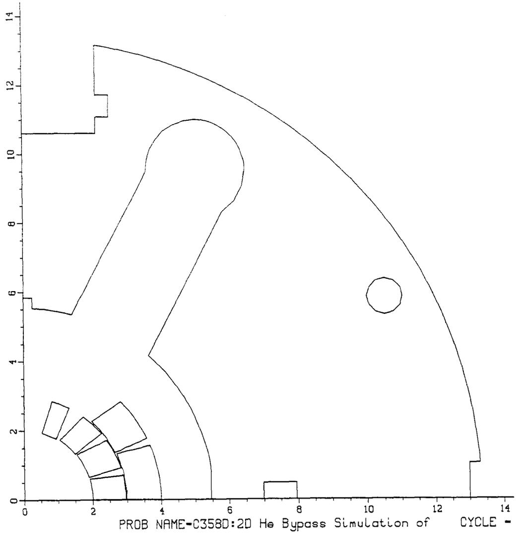
Fig 2. The Geometry of the He bypass lamination.
