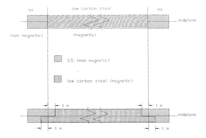
Figure 1: Re-assignment of the location of magnetic and non-magnetic laminations to correct  $a_1$  (skew quadrupole). In SSC 50 mm magnets, a rough estimate shows that moving 1'' of laminations from top to bottom in both ends would fix about one unit of  $a_1$  integrated over the length of the long magnet.
