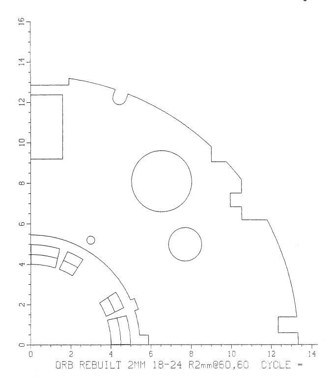
Figure 1: Modified yoke to remove measured  $b_3$  in the arc quadrupoles. A cutout, an additional hole and a missing notch at  $90^{\circ}$  are the proposed modifications.
