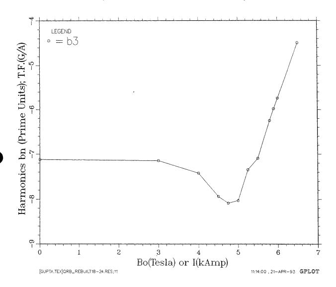
Figure 2: Additional  $b_3$  as a function of current in the arc quadrupoles due to a cutout, a hole and a missing notch.
