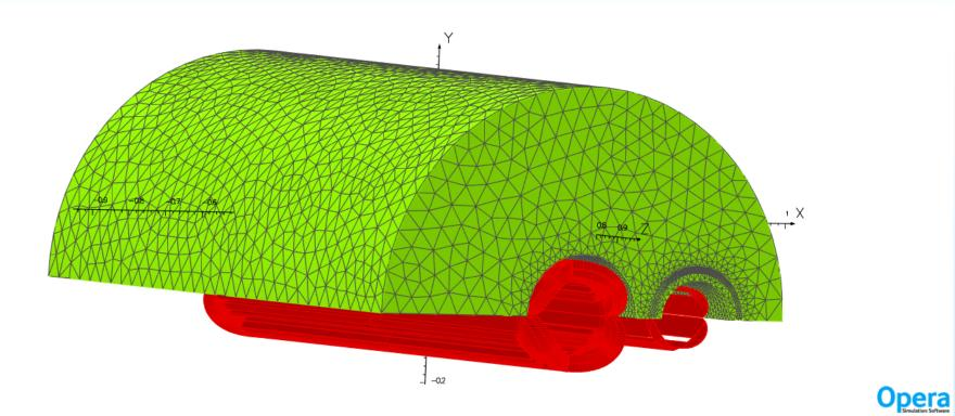
Computer run in progress. For completeness sake, it will be better to use real Q1eF coils, when available (only representative coils used here)
