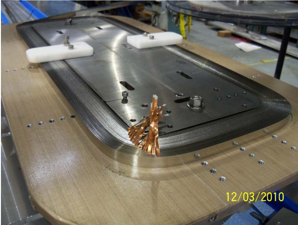
Fig. 4. An FRIB coil during winding.
