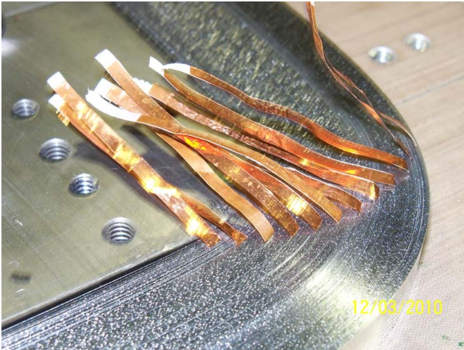
Fig. 5. An FRIB coil with a number of voltage taps.
