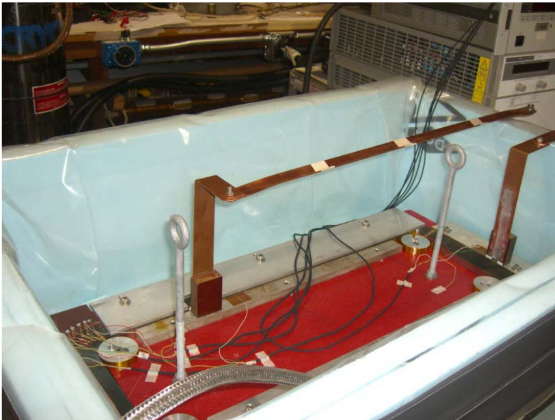
Fig. 9. An FRIB coil being prepared for test in liquid nitrogen at ~77 K.
