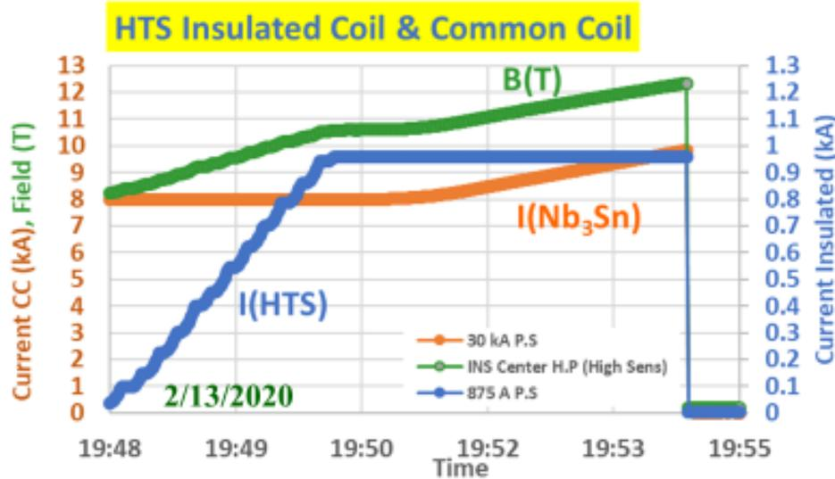
Even though a record 12.3 T hybrid field was obtained, the performance was not limited by HTS coils. It was limited by the Nb<sub>3</sub>Sn coils in every HTS/LTS combination.
