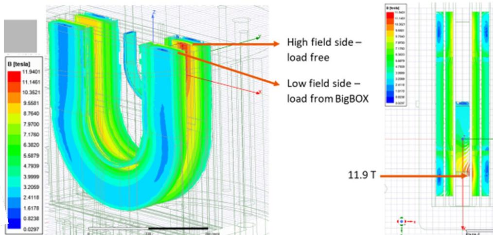
**PSI insert coils had a structure to manage stress concentration**
