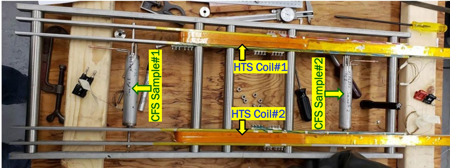
Two HTS coils for testing in field parallel configuration
