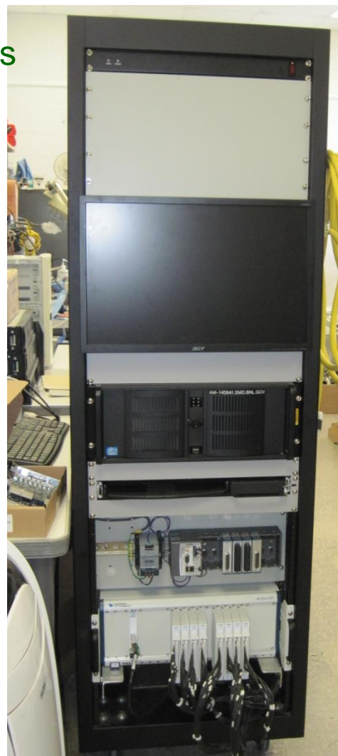
Cabinet #2 (32 channels, 1kV) (expandable to 64 and 3kV)
