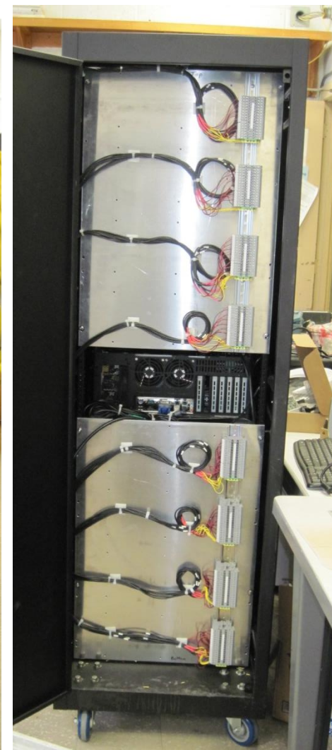
Cabinet #2 (32 channels, 1kV) (expandable to 64 and 3kV)
