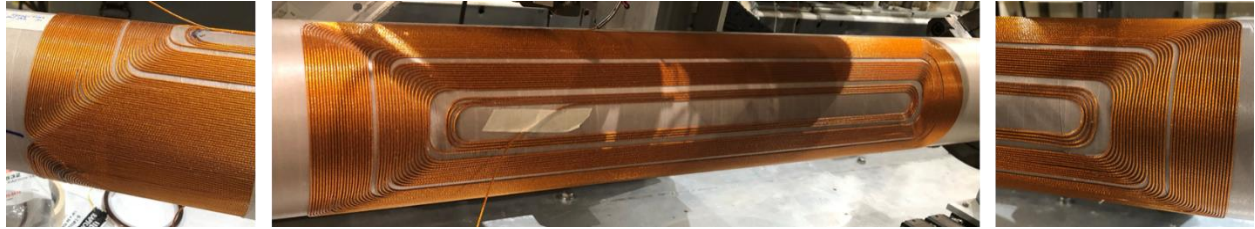
Figure 9: Views of the first layer of the proof-of-principle coil during the winding. The picture on the left shows the left end (where one can also see the midplane turn extending for the full coil length); The picture in the middle shows one half of the full coil and the picture on the right shows the right end.
