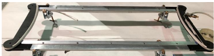
Figure 7.4. Phase I winding of the overpass/underpass coil with a similar Nb_3Sn Rutherford cable that will be used in winding the Phase II coil. Two pictures on the left and right side are views of the same coil turned over to show the other side.
