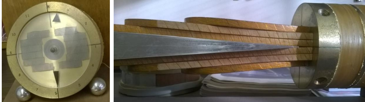
Figure 2.1: Nb_3Sn block coil dipole with cross-section (left) and lifted ends (right).
