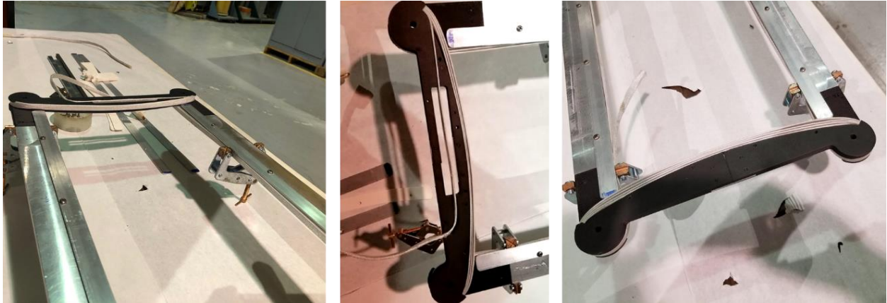
Figure 7.6. More views of the Phase I overpass/underpass coil from different angles.
