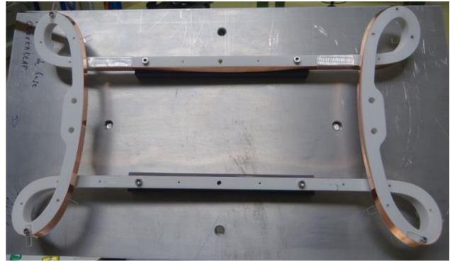
Figure 7.2. Left: Rutherford cable coil wound by the PBL/BNL team in the earlier part of the Phase I proposal with a straight connect between the two overpass/underpass (cloverleaf) sections in the end. Right: HTS tape coil wound by the CERN team with a convex connect between the two cloverleaf (overpass/underpass) sections in the end.
