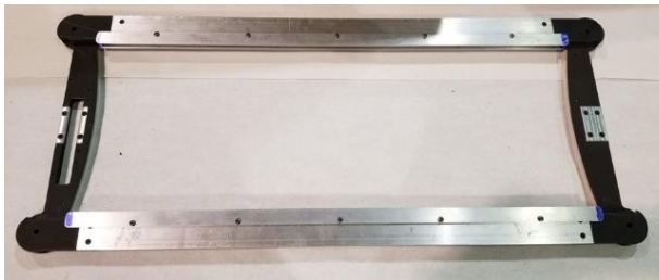
Figure 7.3. Frame for winding the overpass/underpass coil assembled with the printed curved parts (black) and machined straight Aluminum parts (gray). Two pictures on the left and right side are the views of the same frame turned over to show the other side.
