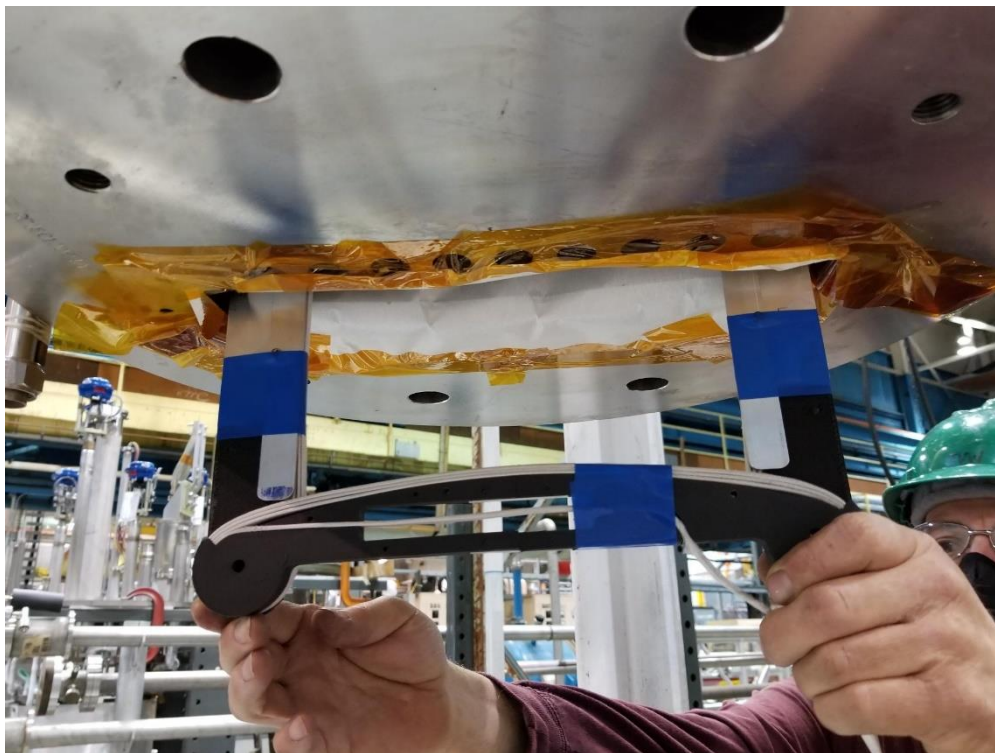
Figure 7.7. A view of the mockup insertion test of the overpass/underpass coil in DCC017.
