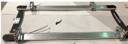
Figure 7.4. Phase I winding of the overpass/underpass coil with a similar Nb_3Sn Rutherford cable that will be used in winding the Phase II coil. Two pictures on the left and right side are views of the same coil turned over to show the other side.
