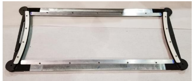
Figure 7.3. Frame for winding the overpass/underpass coil assembled with the printed curved parts (black) and machined straight Aluminum parts (gray). Two pictures on the left and right side are the views of the same frame turned over to show the other side.
