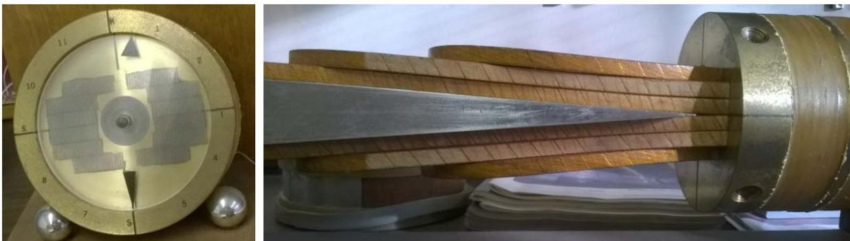
*Figure 1: Nb<sub>3</sub>Sn block coil dipole with cross-section (left) and lifted ends (right).*
