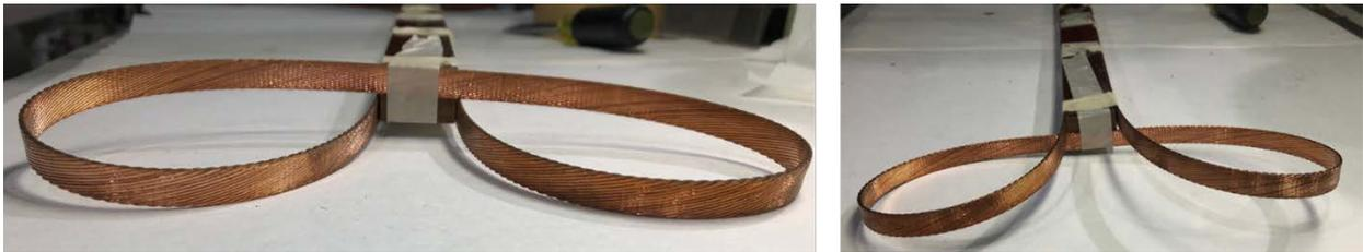
Figure 11: Two views of the winding of a freestanding turn of the overpass/underpass end design with the Rutherford cable.
