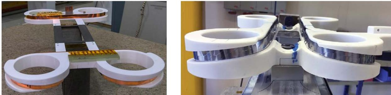
*Figure 7: (left) Winding of an HTS coil at BNL under an SBIR with Energy to Power Solutions, e2P [15], and (right) winding of the practice coils at CERN [9] under EuCARD program.*
