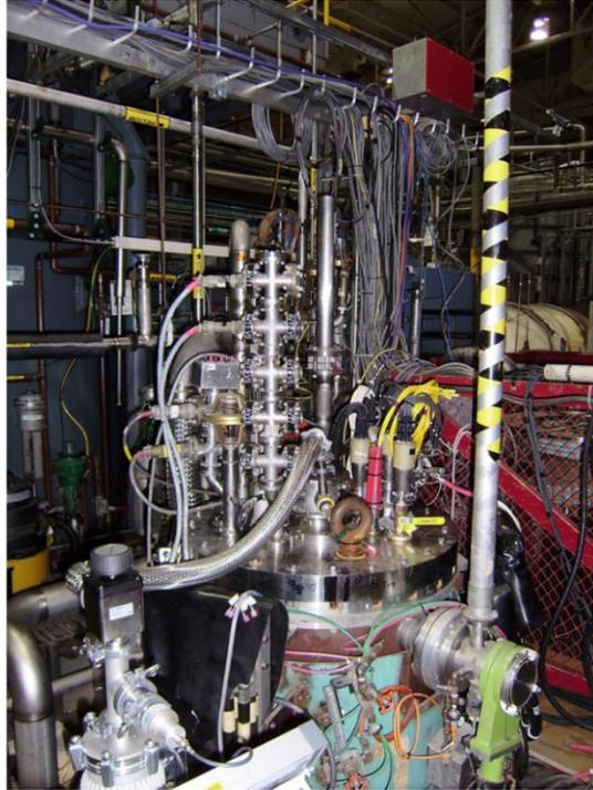
*Fig.8: An HTS magnet in the vertical test Dewar with installed instrumentation. The same test Dewar and a large amount of the same instrumentation will be used during the SMES testing.*
