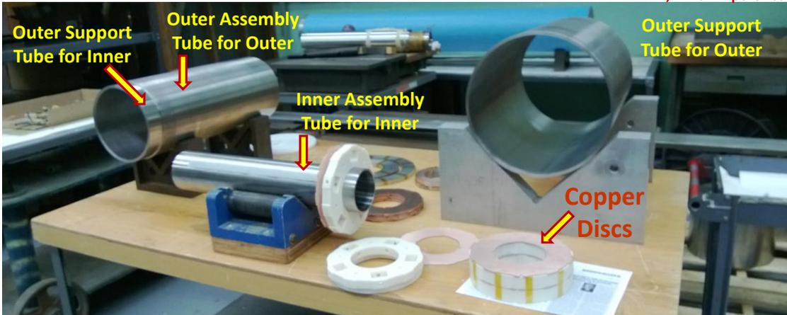
Fig. 5: Various components of high field SMES (coil and support structure).
