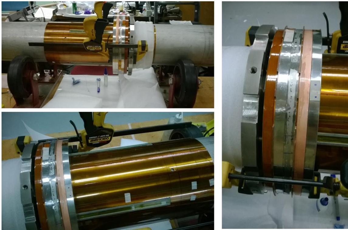
*Fig. 4: Outer coil being assembled with the HTS pancakes on the inner tube of outer assembly.*
