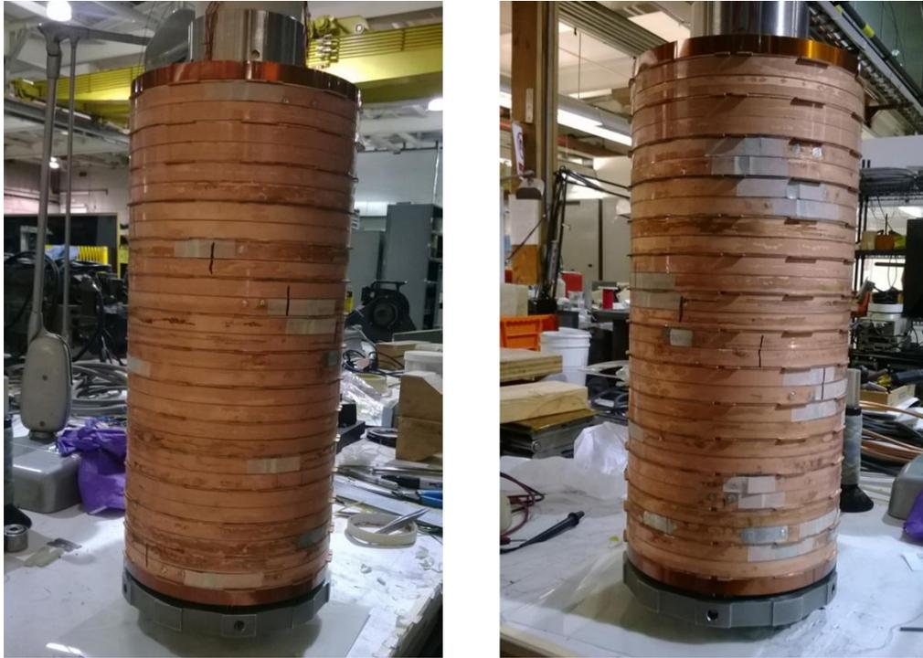
*Fig. 3: Inner coil consisting of all (28) HTS pancakes assembled on the inner tube.*
