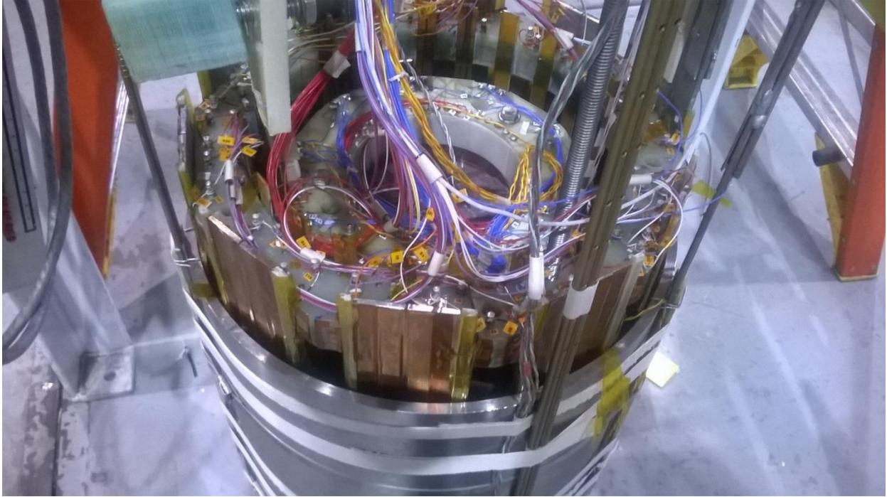
*Figure 3: Instrumentation coming out of the SMES coil.*
