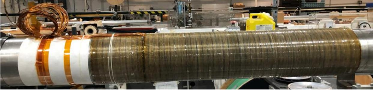
Figure 26: Optimum integral proof-of-principle dipole coil with Fiberglass roving providing necessary pre-tension after the final cure.
