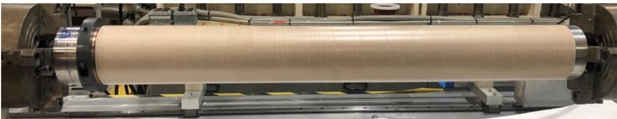
Figure 18: Fiberglass wrap on the Kapton in preparation for winding of the Phase I coil.
