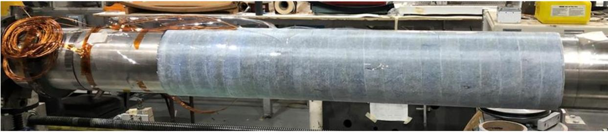
Figure 25: Two layers of coils getting ready for the final cure.
