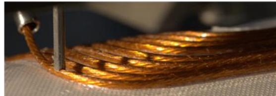
Figure 16: A series of pictures shows more details of the winding of the full-length practice coil. The picture on the bottom right zooms in to show how the superconducting wire is laid and bonded with the ultrasound on the substrate.
