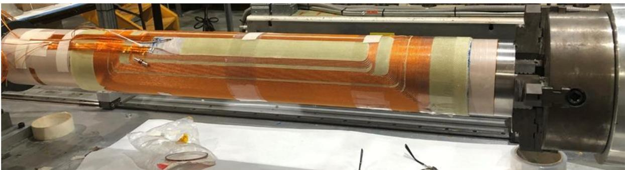
Figure 24: Second layer wound. Voltage-tap wires installed at the start and exit leads.
