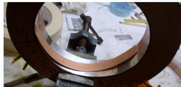
Double pancake coils in test fixture
