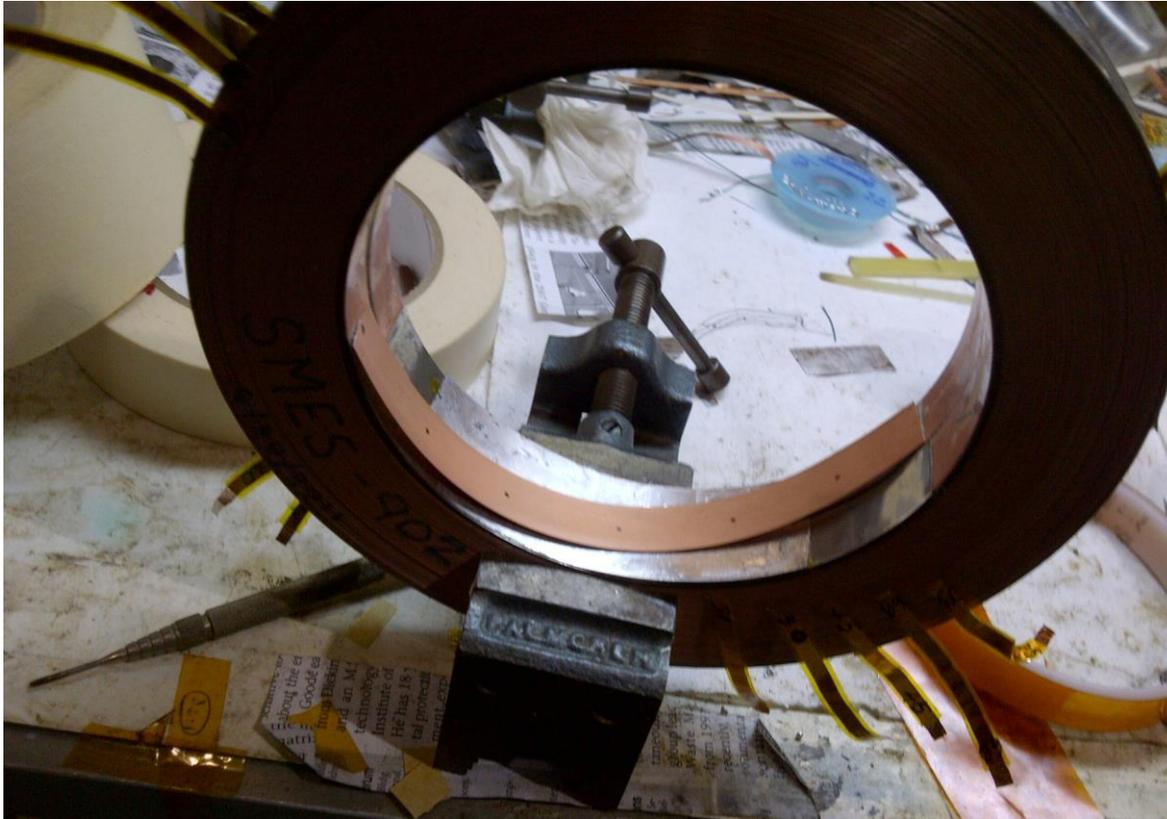
Splice to join two single pancakes to make a double pancake (diagonal splice)
