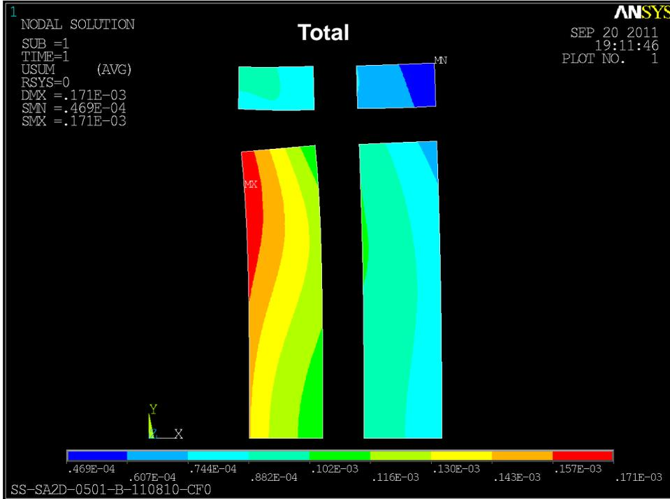
Maximum deformation- 171  $\mu\text{m}$
