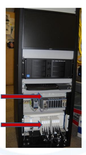
NI FPGA based Quench Detector
