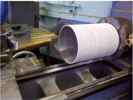
Inner SS tube being machined to size after putting fiberglass epoxy insulation
