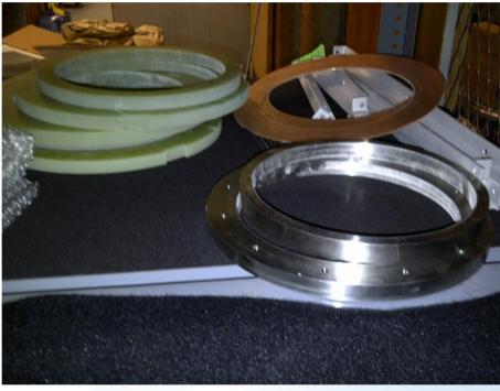
Work in progress. Some more machining and assembly is still needed. The fixture should be ready in December for 77 K double pancake test. A simpler single pancake test fixture was used to qualify construction.
