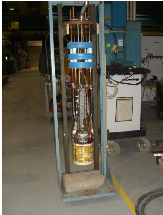
Figure 4.1-8 Photographs of the coil on top-hat with all instrumentation while being prepared for 4 K test.
