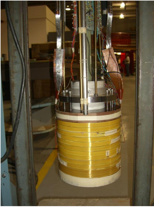
Figure 4.1-8 Photographs of the coil on top-hat with all instrumentation while being prepared for 4 K test.
