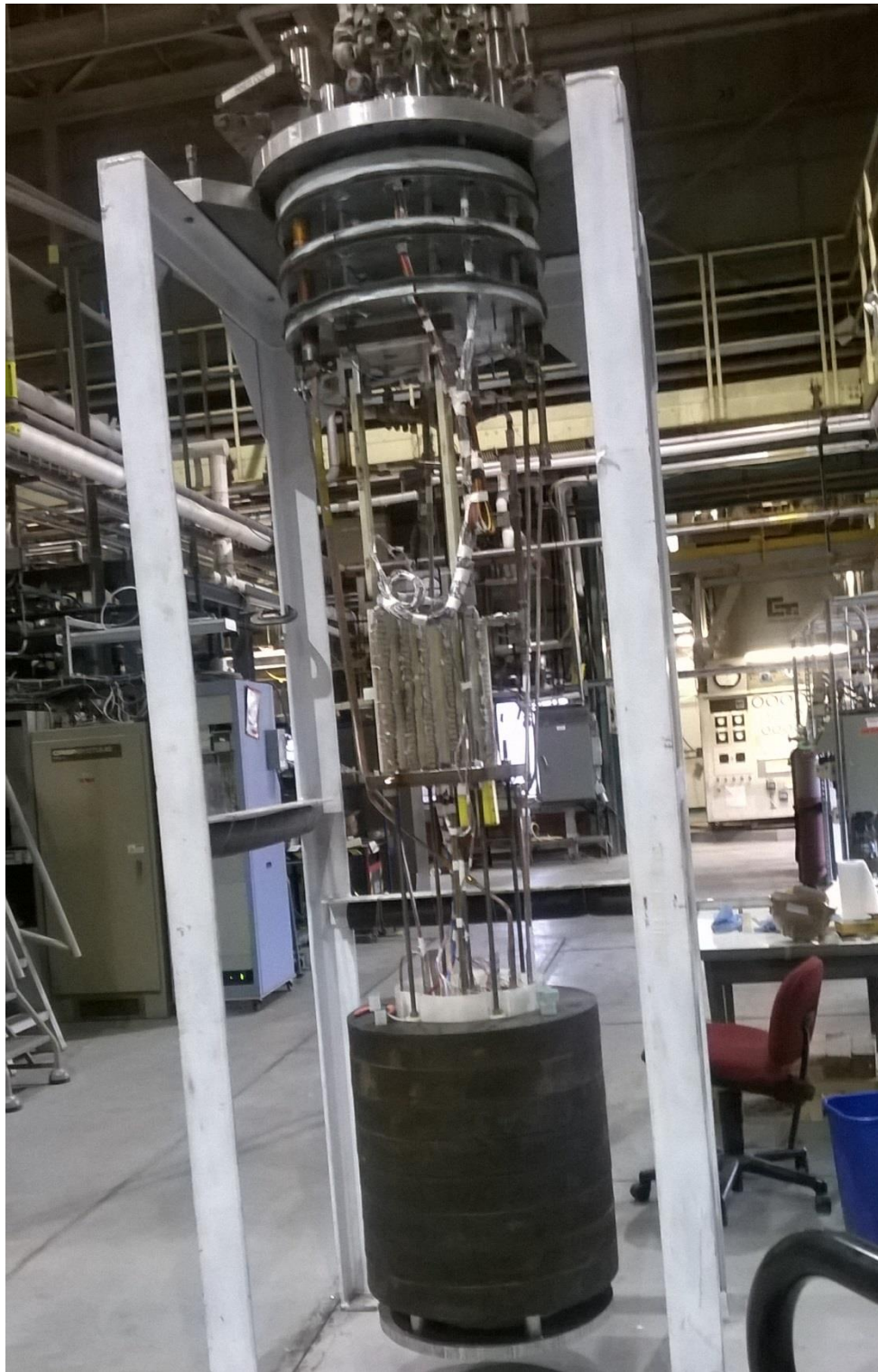
Figure 4.3-5 SMES coil installed on the top hat for testing.
