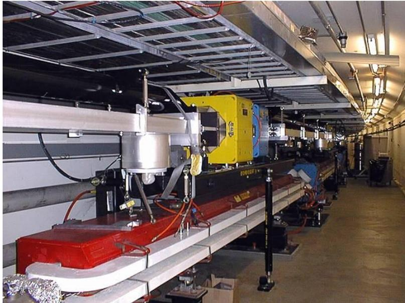
**Figure 29:** The PEP-II collider. The low-energy beam line is mounted above the high-energy beam line. The LER is lowered to the HER elevation in the interaction region.
