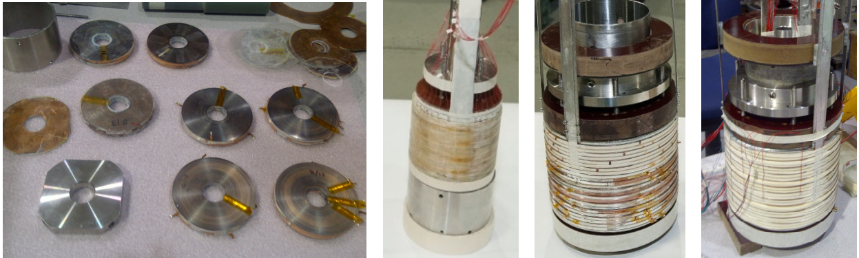
Fig. 1a-d.: High field HTS solenoids built and tested by PBL/BNL collaborations. Left: 25-mm bore pancake coils for insert magnet. Left-center: 7-double-pancake solenoid that generated 16 T. Right-center: Solenoid with 12 double pancakes of 100 mm bore. Right: Nested combination.
