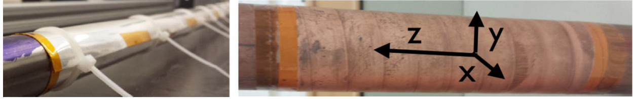
Fig. 9: HTS tape wound around the tube to demonstrate passive superconducting shielding at 77 K. Picture on the left shows two 46 mm wide HTS tapes placed parallel to the tube, and picture on the right shows a 12 mm wide tape wound helically on the tube.
