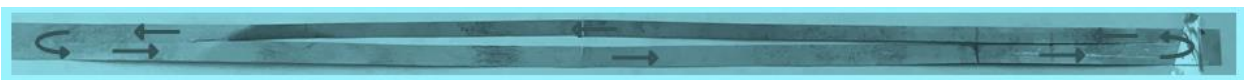
Figure 7: A superconducting tape cut along the length while keeping the two ends intact. A possible path of circulating current to provide shielding is shown.
