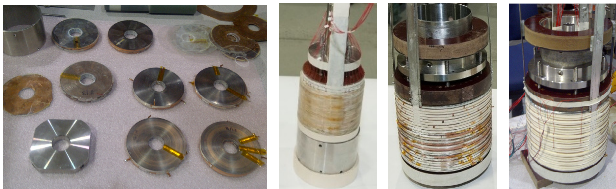
Fig. 1a-d.: High field HTS solenoids built and tested by PBL/BNL collaborations. Left: 25-mm bore pancake coils for insert magnet. Left-center: 7-double-pancake solenoid that generated 16 T. Right-center: Solenoid with 12 double pancakes of 100 mm bore. Right: Nested set.
